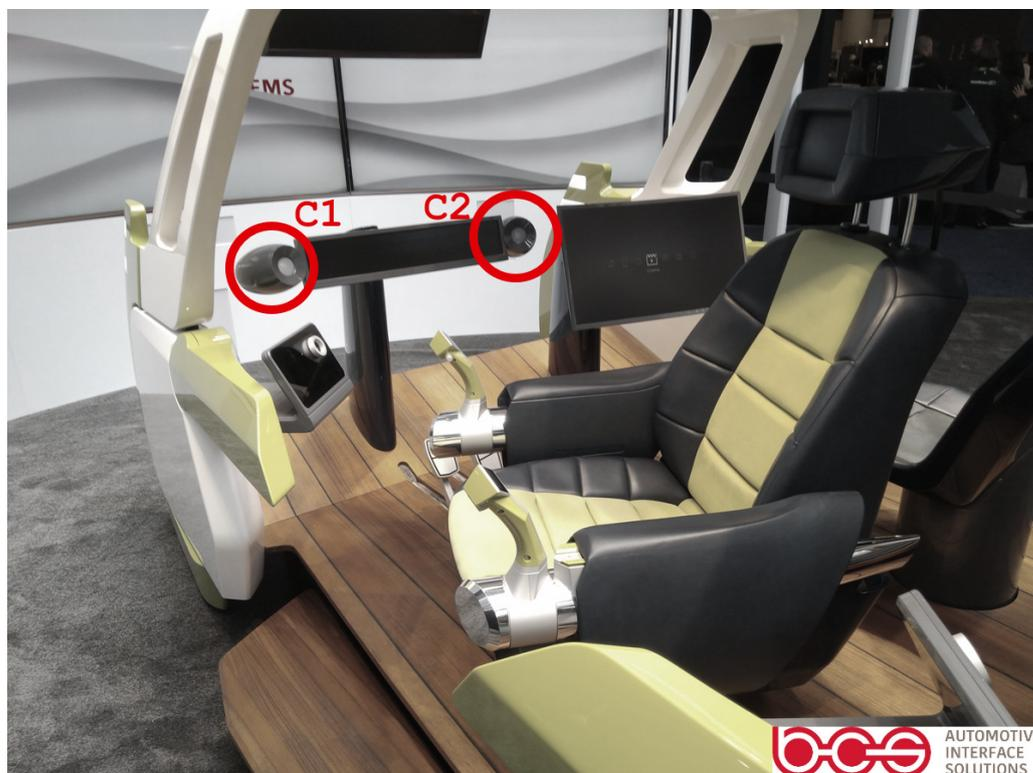
**Figure 1.** Interior of the mockup. The driver's chair currently is in boarding position and at its front the drive sticks are visible. On the co-driver's side the multimedia display is mounted. The front pillar is T-shaped and on its outer sides the IR cameras (s. C1 and C2) are attached behind a polymer film (IR window). (Permission by BCS Automotive Interface Solutions)
