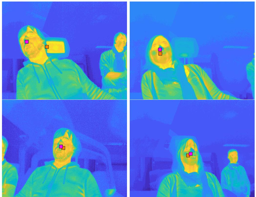
**Figure 8.** Four colormapped LWIR pictures with reference (magenta) and detection (orange) points using the original image size of  $382 \times 288$  pixel. Warm regions are displayed in yellow colour and colder regions are colored blue. In the first picture on the top left the headrest is heated up and the detected point is between the actual head and the heated area. The top left and bottom right picture show examples of people standing in the background.
