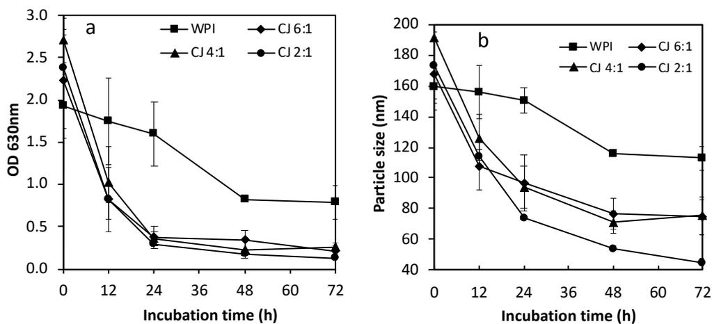
**Figure 4.** Turbidity (a) and particle size (b) of WPI and WPI–inulin conjugate (CJ) solutions (6% *w/w* protein concentrate, pH 6.00) after heating at 85 °C. WPI and CJ were incubated at 80 °C (no RH control) for 0–72 h. Here, 6:1, 4:1 and 2:1 refer to the weight ratios of WPI to inulin. Error bars are standard deviations.
