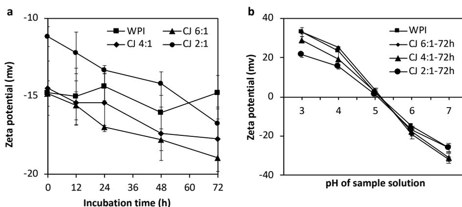
**Figure 5.** (a) Effect of incubation time on zeta potentials of WPI and CJ (2:1, 4:1, and 6:1 WPI–inulin) solutions (6% w/w, pH 6) after heating at 85 °C. (b) Zeta potentials of heated WPI and CJ solutions as a function of pH. Error bars are standard deviations from triplicate measurements.
