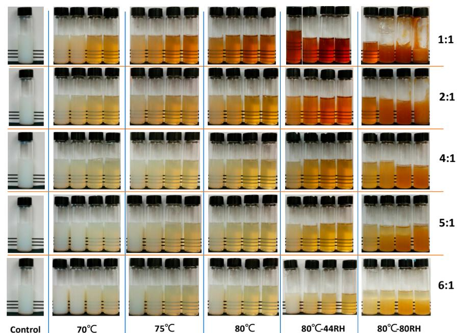
**Figure 1.** Solutions (6% *w/w* protein, pH 6.00) of whey protein isolate (WPI)–inulin mixtures (e.g., control) or conjugates prepared in different dry-heating conditions after heating at 85 °C for 15 min. Samples from top to bottom were at different WPI to inulin ratios. Vials from left to right at the same dry-heating temperature represent conjugates at 12, 24, 48, and 72 h incubation time.
