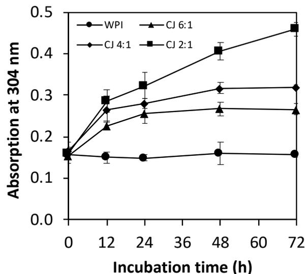
**Figure 2.** Formation of Amadori compounds monitored at 304 nm in WPI and WPI–inulin conjugates (CJ). WPI and CJ (6:1, 4:1 and 2:1 weight ratio (WR) of WPI to inulin) were incubated at 80 °C (no relative humidity (RH) control) for 0–72 h. All samples were prepared to contain 2.5 mg/mL protein. Error bars are standard deviations from triplicate measurements.
