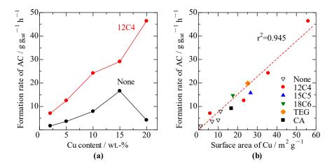
**Figure 5.** Effect of Cu content (**a**) and  $SA_{Cu}$  (**b**) on formation rate of AC at 200 °C.
