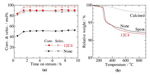
**Figure 6.** Catalytic performance at 260 °C and a W/F of 0.080 h over none- and 12C4-10Cu/SiO<sub>2</sub> (**a**) and TG profiles of the spent none-, spent 12C4-, and calcined none-10Cu/SiO<sub>2</sub> catalysts (**b**).
