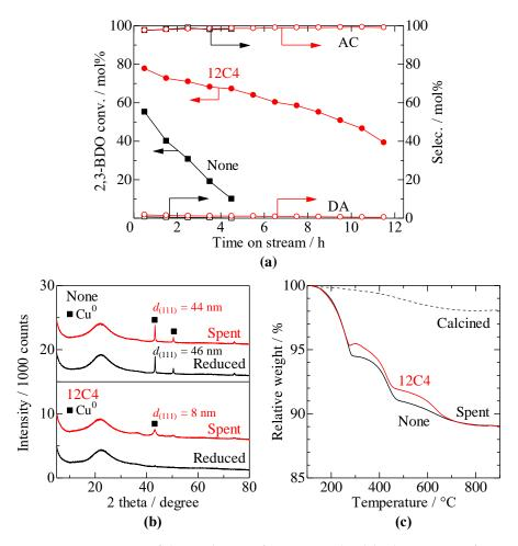
**Figure 4.** Time course of the catalytic performance in the dehydrogenation of 2,3-BDO at 200 °C and a W/F of 0.14 h over none- and 12C4-10Cu/SiO<sub>2</sub> catalysts (**a**), XRD patterns of reduced and spent 10Cu/SiO<sub>2</sub> catalysts (**b**), and TG profiles of the spent none-, spent 12C4-, and calcined none-10Cu/SiO<sub>2</sub> catalysts (**c**).
