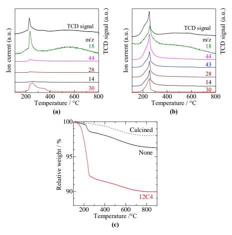
**Figure 1.** TD-MS profiles of the as-prepared none- (**a**) and 12C4-2Cu/SiO<sub>2</sub> (**b**) and TG curves of the as-prepared none-, as-prepared 12C4-, and calcined none-2Cu/SiO<sub>2</sub> (**c**).
