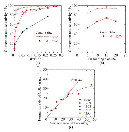
**Figure 7.** Effect of contact time, W/F, in the dehydrogenation of 1,4-BDO to GBL over  $10Cu/SiO_2$  catalyst at 260 °C (**a**), effect of Cu content at 240 °C and W/F = 0.054 h (**b**), and relation between Cu surface area on formation rate of GBL at 240 °C (**c**).
