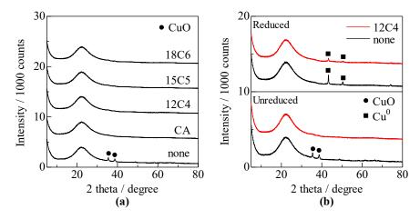
**Figure 2.** XRD profiles of 2Cu/SiO<sub>2</sub> catalysts prepared with different organic additives before reduction (**a**) and none- and 12C4-2Cu/SiO<sub>2</sub> catalysts (**b**).
