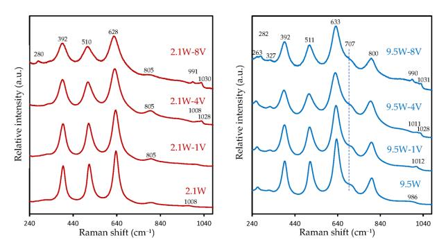
**Figure 6.** Raman spectra recorded on V<sub>2</sub>O<sub>5</sub>-WO<sub>3</sub>/TiO<sub>2</sub> catalysts calcined in air at 450 °C.
