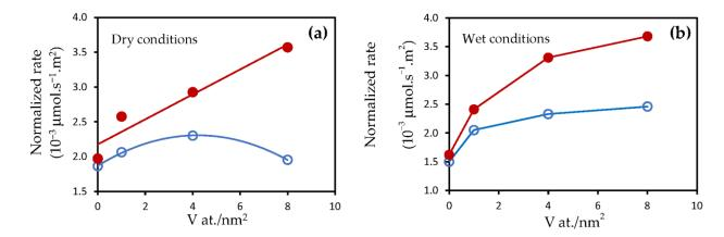
**Figure 4.** Vanadium density and relative concentration of vanadium dependencies of the normalized reaction rate of 2.1W-xV ( $\bigcirc$ ) and 9.5W-xV ( $\bullet$ ) in ammonia-SCR: 400 ppm NO, 400 ppm NH<sub>3</sub>, 8 vol.% O<sub>2</sub> in the presence (wet conditions) or in the absence (dry conditions) of 10 vol.% H<sub>2</sub>O: (**a**) dry conditions; (**b**) wet conditions.
