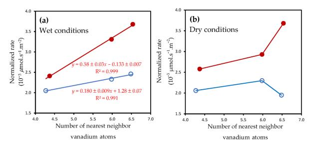
**Figure 11.** Dependency of the nearest vanadium atoms in  $VO_x$  clusters on the normalized reaction rates measured on 2.1W-xV ( $\odot$ ) and 9.5W-xV ( $\bullet$ ) exposed at 160 °C to 400 ppm NO, 400 ppm NH<sub>3</sub>, 8 vol.% O<sub>2</sub> in the presence (**a**) and in the absence of 10 vol.% H<sub>2</sub>O (**b**).
