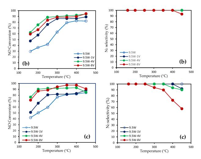
**Figure 3.** Conversion and  $N_2$  selectivity profiles vs. temperature recorded on 9.5W-xV during ammonia SCR: (a) Dry ID 2 operating conditions on preheated freshly prepared samples; (b) Wet conditions ID 3; (c) Dry conditions ID 2 on samples exposed to wet conditions according to ID3. Gas hourly space velocity of 75,000 mL.h<sup>-1</sup>.g<sup>-1</sup>.
