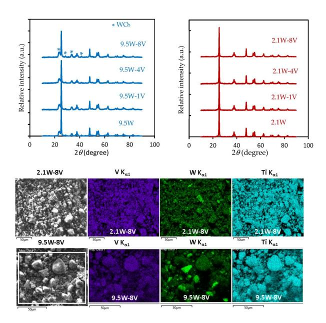
**Figure 5.** XRD and EDS analyses on freshly prepared  $V_2O_5$ -WO<sub>3</sub>/TiO<sub>2</sub> catalysts calcined in air at 450 °C. 3.3.2. Raman Spectroscopy
