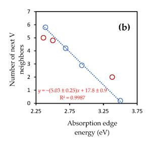
**Figure 7.** UV-vis spectra recorded for the series 2.1W-xV (**a**) and relationship between the estimated absorption edge value from (**a**) and the number of next V neighbors in VO<sub>x</sub> clusters (**b**). Red circle data from reference [27], blue circle data from reference [28].
