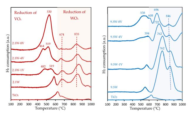
Figure 8.  $H_2$ -consumption profiles vs. temperature from  $H_2$ -TPR experiments for calcined  $V_2O_5$ - $WO_3/TiO_2$  SCR-catalysts.
