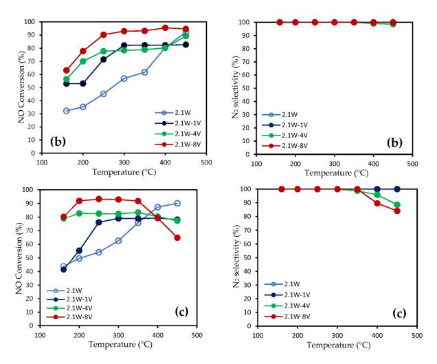
**Figure 2.** Conversion and  $N_2$  selectivity profiles vs. temperature recorded on 2.1W-xV during ammonia SCR: (a) Dry ID 2 operating conditions on preheated freshly prepared samples; (b) Wet conditions ID 3; (c) Dry conditions ID 2 on samples exposed to wet conditions according to ID3. Gas hourly space velocity of 75,000 mL.h<sup>-1</sup>.g<sup>-1</sup>.
