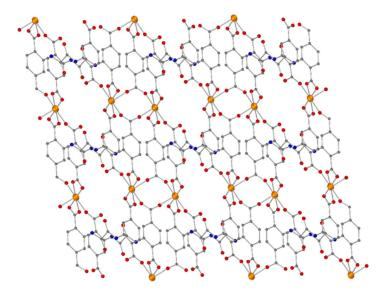
**Figure 1.** The 3D framework of the **3D-Fe-MOF** down to the *a* axis. Color code: Fe orange, C, grey, H cyan, O red, N blue.
