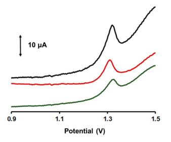
**Figure 5.** Background-subtracted DP voltammograms for GLU concentrations in the range of  $100-300 \mu$ M in phosphate buffer 0.1 M, pH 6 obtained with the modified GPE.
