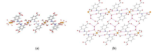
**Figure 3.** Two views of the 2D framework of **2D-Fe-MOF**. (a) A single layer down to the *b* axis and (b) two neighboring layers down to *b* axis showing the intra- and inter-layer hydrogen bonding (purple dashed lines). Color code: Fe orange, *C*, grey, H cyan, O red, N blue.
