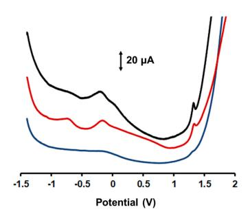
**Figure 4.** DP voltammograms of 0.6 mM GLU in 0.10 M phosphate buffer, pH 6.0 at the modified GPEs loaded with 1% (black line), 2% (red line), and 5% (blue line) w/w **3D-Fe-MOF**.
