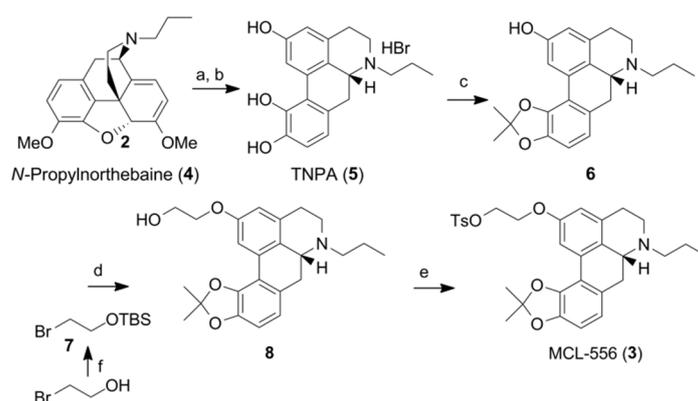
**Scheme 2.** Synthesis of precursor MCL-556 (**3**). Reagents and conditions: (a) *i.* DIAD, MeCN, heat; *ii.* MeOH, EtOAc; (b) 48% HBr/AcOH, 120 °C; (c) CH<sub>3</sub>COCH<sub>3</sub>, P<sub>2</sub>O<sub>5</sub>, THF, 60 °C; (d) **7**, 5 N NaOH, THF, 70 °C; (e) Ts<sub>2</sub>O, Et<sub>3</sub>N, DMAP, CH<sub>2</sub>Cl<sub>2</sub>; (f) TBSCl, Et<sub>3</sub>N, CH<sub>2</sub>Cl<sub>2</sub>.
