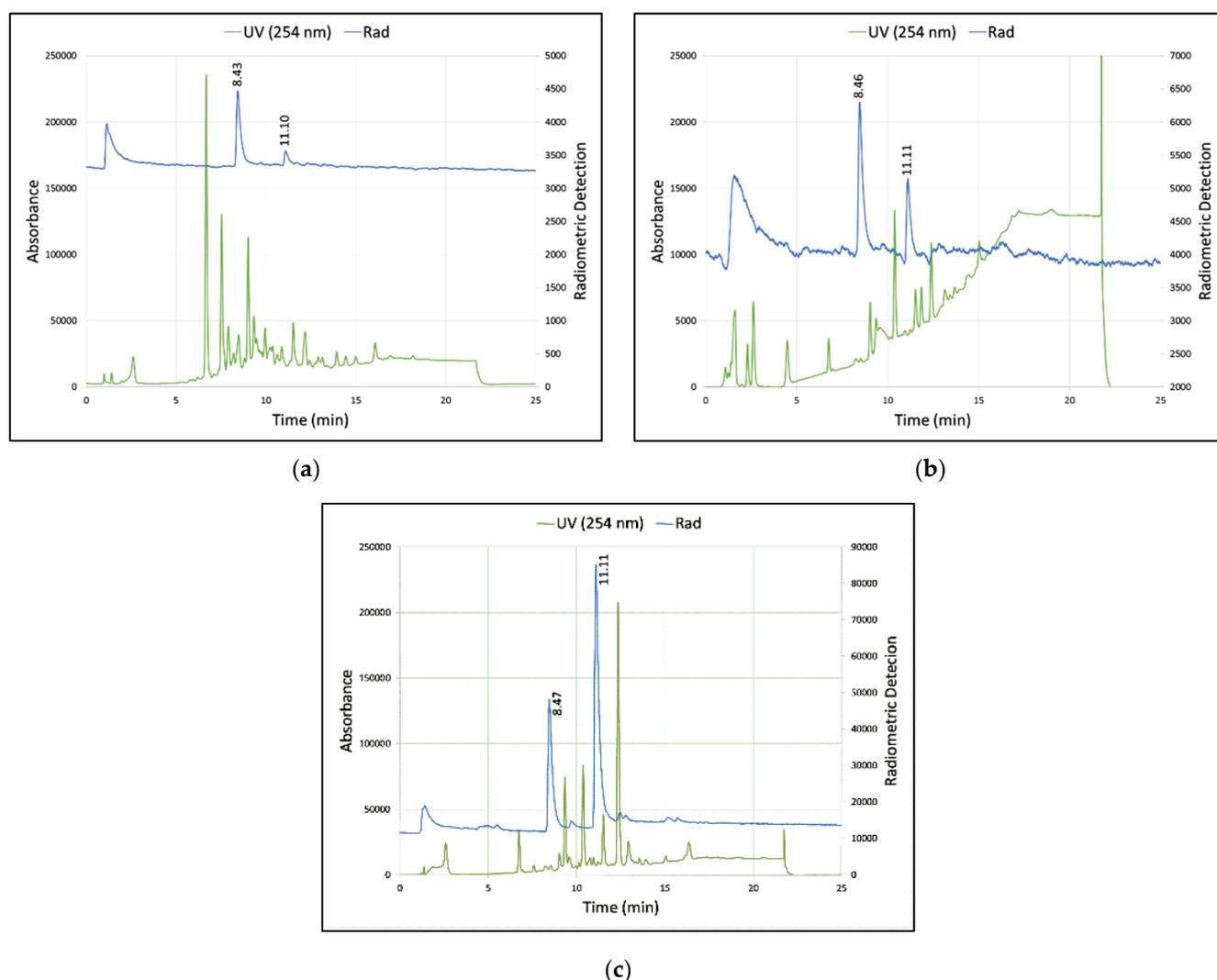
**Figure 3.** Representative radio-HPLCs of catechol deprotection reactions using: (a) 6 N H<sub>2</sub>SO<sub>4</sub> (Table 1, Entry 2); (b) 90% TFA (Table 1, Entry 4); (c) In(OTf)<sub>3</sub> (Table 1, Entry 3)). [<sup>18</sup>F]2 = ~11.1 min. [<sup>18</sup>F]1 = ~8.4 min. See the Supporting Information for HPLC conditions (HPLC 1, Program A).
