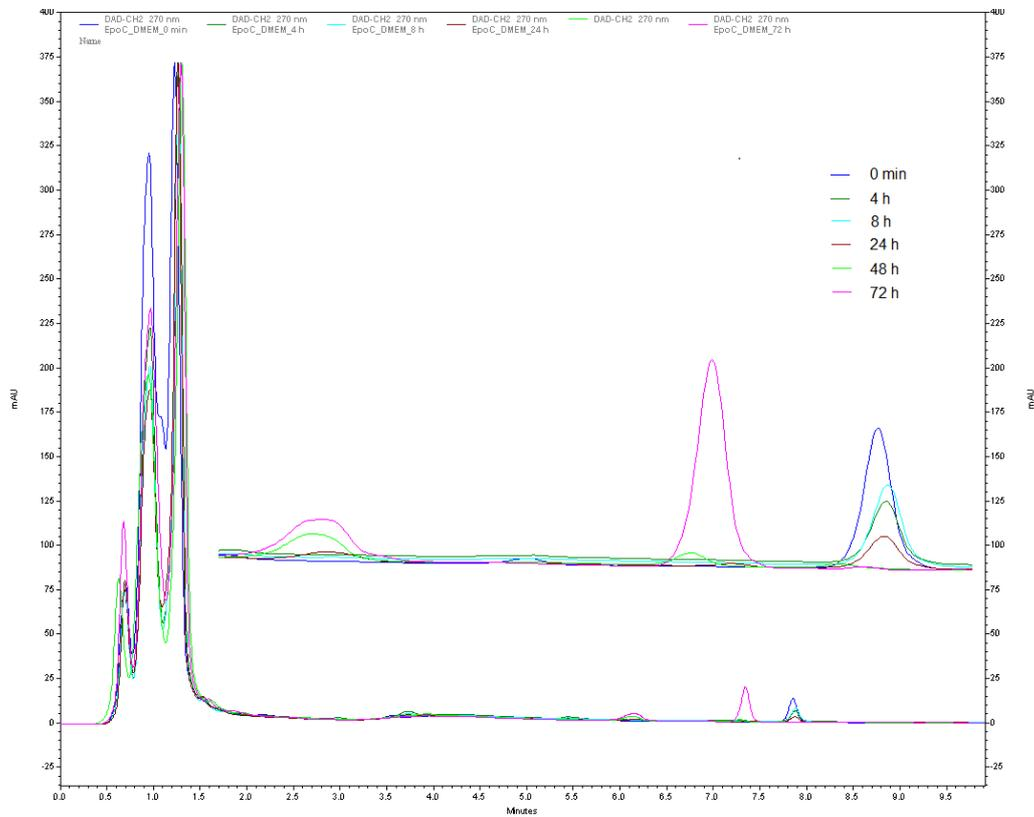
**Figure S6:** Stability of Epo C in DMEM over a 24 h time period. HPLC traces obtained with a Waters Symmetry C18 3.5  $\mu\text{m}$ , 4.6x100 mm column. Elution method: Gradient from 60:40 to 80:20 ACN/H<sub>2</sub>O within 12 min, flow rate: 1 mL/min. Detection at 250 nm.
