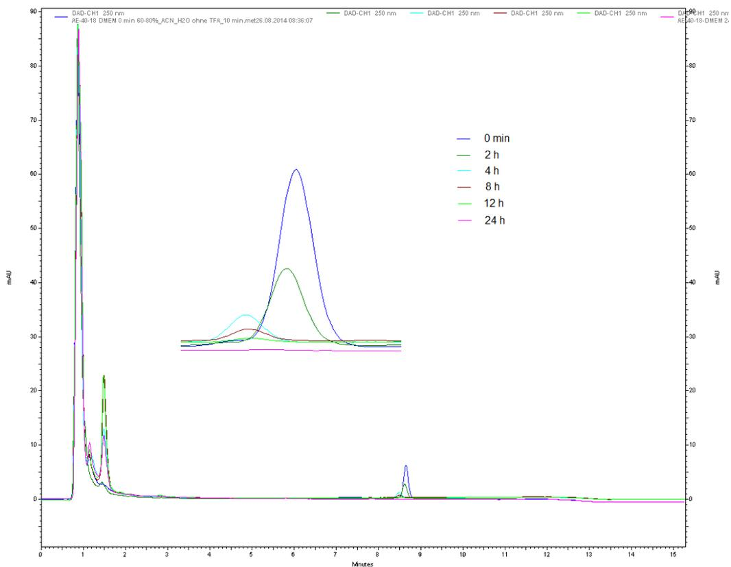
**Figure S4:** Stability of deaza-Epo C (**5**) in DMEM over a 24 h time period. HPLC traces obtained with a Waters Symmetry C18 3.5  $\mu$ m, 4.6x100 mm column. Elution method: Gradient from 60:40 to 80:20 ACN/H<sub>2</sub>O within 12 min, flow rate: 1 mL/min. Detection at 250 nm.
