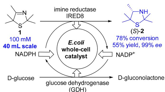
**Scheme 2.** Biocatalytic enantioselective reduction of 3-thiazoline **1** to (S)-**2** by means of an *E. coli* whole-cell catalyst bearing the imine reductase IRED8 from *Mycobacterium smegmatis* and glucose dehydrogenase from *Bacillus subtilis*.
