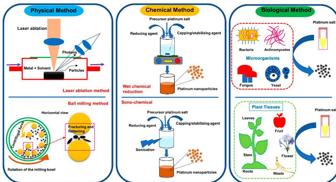
**Figure 2.** Synthesis of platinum nanoparticles through various methods.
