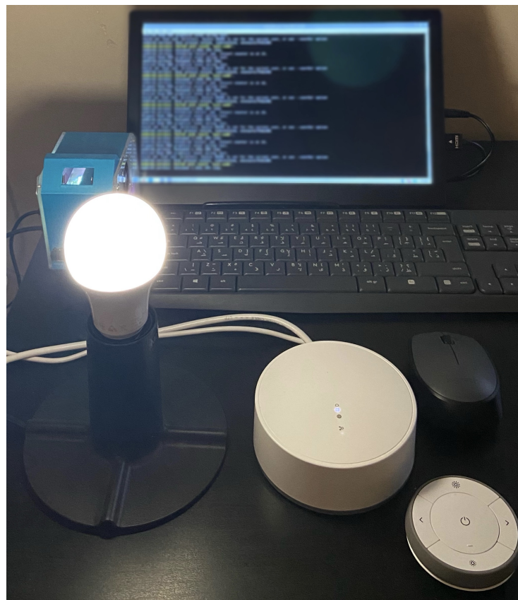
Figure 3. Photo of experimental setup showing Raspberry Pi, Smart Bulb, TRÅDFRI Gateway, and Remote Control.
