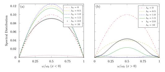
**Figure 3.** The spectral distribution of particles created on the two sides of a moving  $\delta - \delta'$  mirror as a function of  $\omega/\omega_0$  for different values of  $\lambda_0$ , with  $\mu_0 = 1$ : (a) the plot of  $(\epsilon^2 \tau/\pi)^{-1} \times dN_-/d\omega$ ; (b) the plot of  $(\epsilon^2 \tau/\pi)^{-1} \times dN_+/d\omega$ . See text for details. Figure is generated from results within Ref. [46].
