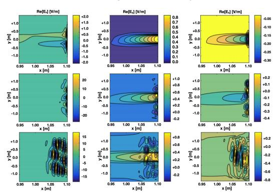
**Figure 3.** Real parts of the electric field components,  $E_x$  (radial; **left**),  $E_y$  (poloidal; **middle column**), and  $E_z$  (toroidal; **right**) for a density of  $10^{19}/\text{m}^3$  (**top**),  $5 \times 10^{18}/\text{m}^3$  (**middle row**), and  $10^{18}/\text{m}^3$  (**bottom**) at the last closed flux surface with a magnetic field tilt of  $\Theta = 0.2$  rad.  $E_y = 1$  V/m was imposed as "antenna" at the antenna location.
