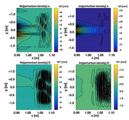
**Figure 7.** Perturbed density of the electrons, e (**top**), and deuterons, D (**bottom**), corresponding to the electric field shown in the bottom of Figure 3.
