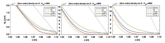
**Figure 9.** Zero-order density at five poloidal positions (bottom, 1/4 up, middle, 3/4 up, and top) for  $P_{RF} = 0$  (**left**),  $P_{RF} = 3$  MW (**middle**), and  $P_{RF} = 5$  MW (**right**). The grey dotted line is the density variation in absence of RF power according to the simplified model adopted.
