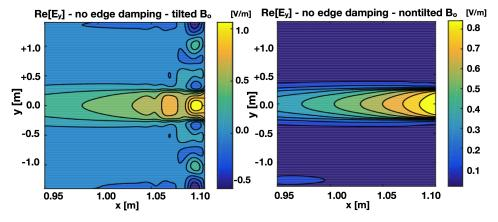
**Figure 4.** Poloidal component in absence of poloidal edge damping (**left**) and in absence of the antenna tilt (**right**);  $E_V = 1 \text{ V/m}$  at the antenna location.
