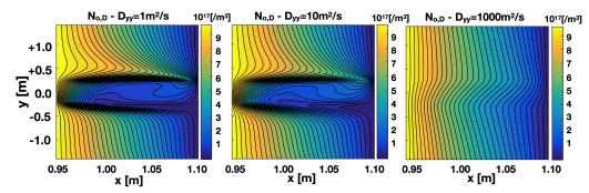
**Figure 8.** RF corrected zero-order density for very low (1 m<sup>2</sup>/s; **left**), low (10 m<sup>2</sup>/s; **middle**), and moderately high (1000 m<sup>2</sup>/s; **right**) parallel diffusion for parameters corresponding to the electric field shown in the bottom plots of Figure 3.
