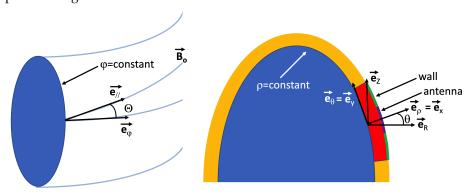
Figure 2. Sketch of the considered geometry. In the slab geometry adopted for the computations,  $\vec{e}_x = \vec{e}_\rho$  and  $\vec{e}_y = \vec{e}_\theta$ . The poloidal middle of the antenna is identified with y = 0. See text for details.
