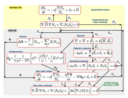
**Figure 1.** Scheme for modelling wave–plasma interaction. Note that at the outset when the radio frequency (RF) power,  $P_{RF} = 0$ , charge neutrality is assumed, so that not only the ponderomotive but also the electrostatic potential is assumed to be zero.
