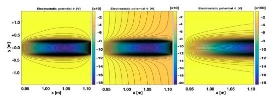
**Figure 6.** Electrostatic potential consistent with a local charge neutrality imbalance near the antenna of  $10^{14}/\text{m}^3$ :  $\Phi_{\text{antenna}} = 0$  (**left**),  $\Phi_{\text{antenna}} = -35 \text{ V}$  (**middle**), and  $\partial \Phi_{\text{antenna}}/\partial x = 0$  (**right**). See text for details.
