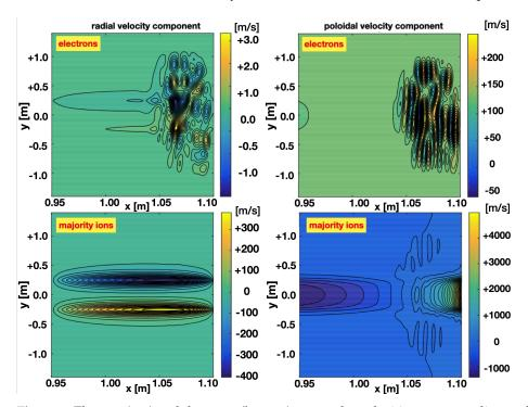
**Figure 5.** Electron (**top**) and deuteron (**bottom**) zero-order velocities corresponding to the electric field in the bottom of Figure 3.
