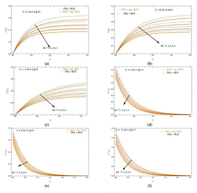
**Figure 4.** The axial,  $F(\eta)$ , and transverse,  $F'(\eta)$ , velocities versus the similarity variable,  $\eta$ , for various values of  $Da^{-1}$  and Q = M = 1. (a) F(n), for  $V_c = 1$ , (b) F(n), for  $V_c = 0$ , (c) F(n), for  $V_c = -1$ , (d) F'(n), for  $V_c = 1$ , (e) F'(n), for  $V_c = 0$ , and (f) F'(n), for  $V_c = -1$ . The orange solid line refers to the (TiO<sub>2</sub>-Ag, H<sub>2</sub>O) HNF and dotted line to (TiO<sub>2</sub>, H<sub>2</sub>O).
