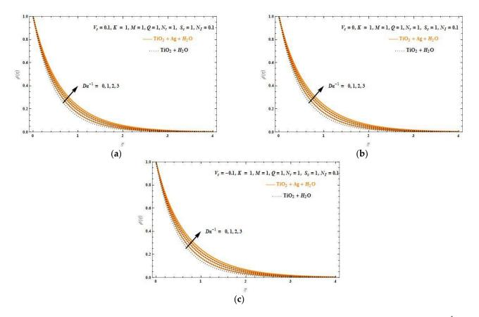
**Figure 15.** Concentration profiles,  $\phi(\eta)$ , versus similarity variable,  $\eta$ , for various  $Da^{-1}$  values,  $S_c = N_r = M = Q = K = 1$ ,  $N_I = 0.1$ , and (a)  $V_c = 0.1$ , (b)  $V_c = 0$ , and (c)  $V_c = -0.1$ .
