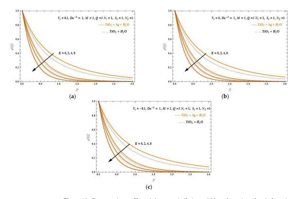
**Figure 13.** Concentration profiles,  $\phi(\eta)$ , versus similarity variable,  $\eta$ , for various chemical reaction coefficient, K, values,  $Da^{-1} = N_I = N_r = M = Q = S_c = 1$ , and (a)  $V_c = 0.1$ , (b)  $V_c = 0$ , and (c)  $V_c = -0.1$ .
