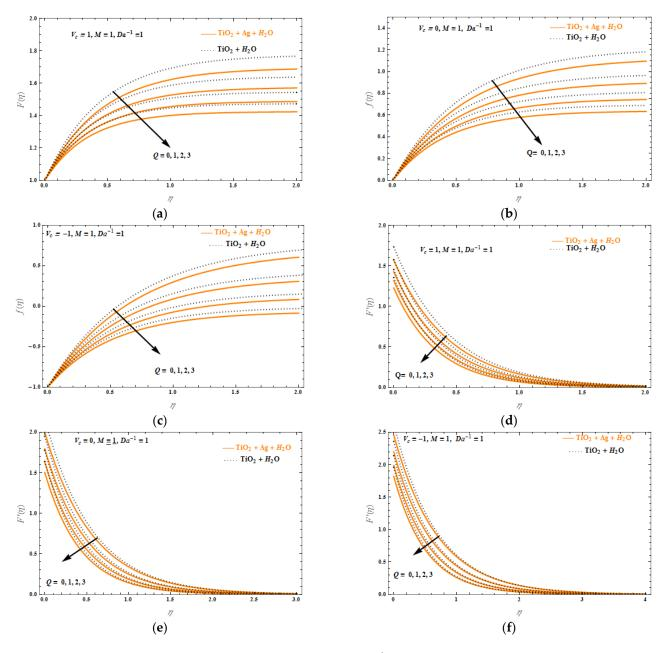
**Figure 6.** The axial,  $F(\eta)$ , and transverse,  $F'(\eta)$ , velocities versus the similarity variable,  $\eta$ , for various values of Q and  $M = Da^{-1} = 1$ . (a) F(n), for  $V_c = 1$ , (b) F(n), for  $V_c = 0$ , (c) F(n), for  $V_c = -1$ , (d) F'(n), for  $V_c = 1$ , (e) F'(n), for  $V_c = 0$ , and (f) F'(n), for  $V_c = -1$ . The orange solid line refers to the (TiO<sub>2</sub>-Ag, H<sub>2</sub>0) HNF and dotted line to (TiO<sub>2</sub>, H<sub>2</sub>O).
