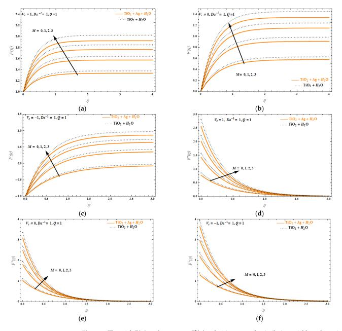
**Figure 5.** The axial,  $F(\eta)$ , and transverse,  $F'(\eta)$ , velocities versus the similarity variable,  $\eta$ , for various values of M and  $Q = Da^{-1} = 1$ . (a) F(n), for  $V_c = 1$ , (b) F(n), for  $V_c = 0$ , (c) F(n), for  $V_c = -1$ , (d) F'(n), for  $V_c = 1$ , (e) F'(n), for  $V_c = 0$ , and (f) F'(n), for  $V_c = -1$ . The orange solid line refers to the (TiO<sub>2</sub>-Ag, H<sub>2</sub>O) HNF and dotted line to (TiO<sub>2</sub>, H<sub>2</sub>O).
