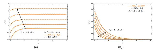
**Figure 8.** (a) Axial,  $F(\eta)$ , and (b) transverse,  $F'(\eta)$ , velocities versus the similarity variable,  $\eta$ . M = Q = 1,  $Da^{-1} = 2$ . The orange solid line refers to the (TiO<sub>2</sub>-Ag, H<sub>2</sub>O) HNF and dotted line to (TiO<sub>2</sub>, H<sub>2</sub>O).
