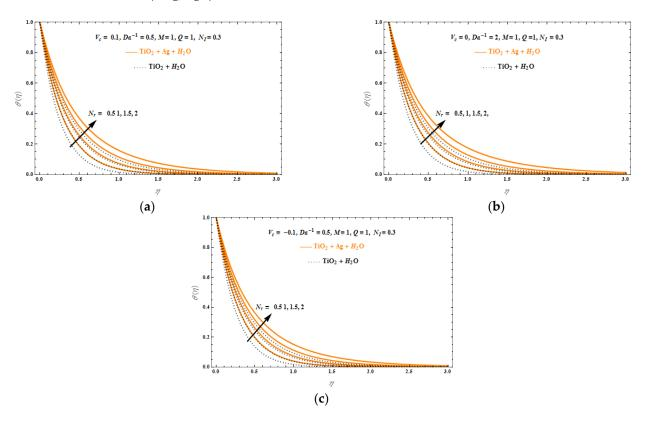
**Figure 9.** Temperature profiles,  $\theta(\eta)$ , versus similarity variable,  $\eta$ , for various thermal radiation parameter,  $N_r$ , values,  $Da^{-1} = 0.5$ ,  $N_I = 0.3$ , and M = Q = 1, and (a)  $V_c = 0.1$ , (b)  $V_c = 0$ , and (c)  $V_c = -0.1$ .
