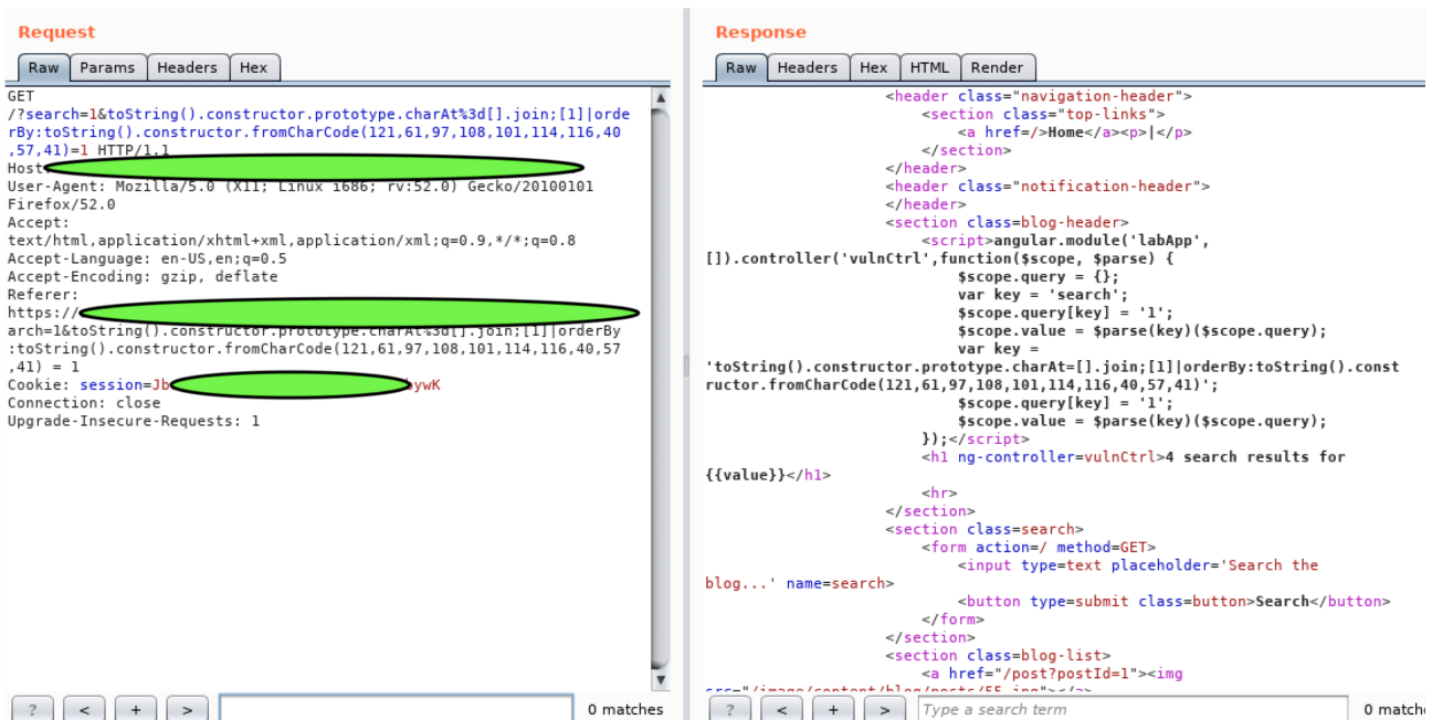
Figure 4. Escaping AngularJS framework using fromCharCode conversion.
