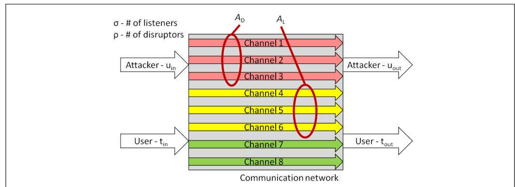
**Figure 1.** A network configuration with multiple possible channels.
