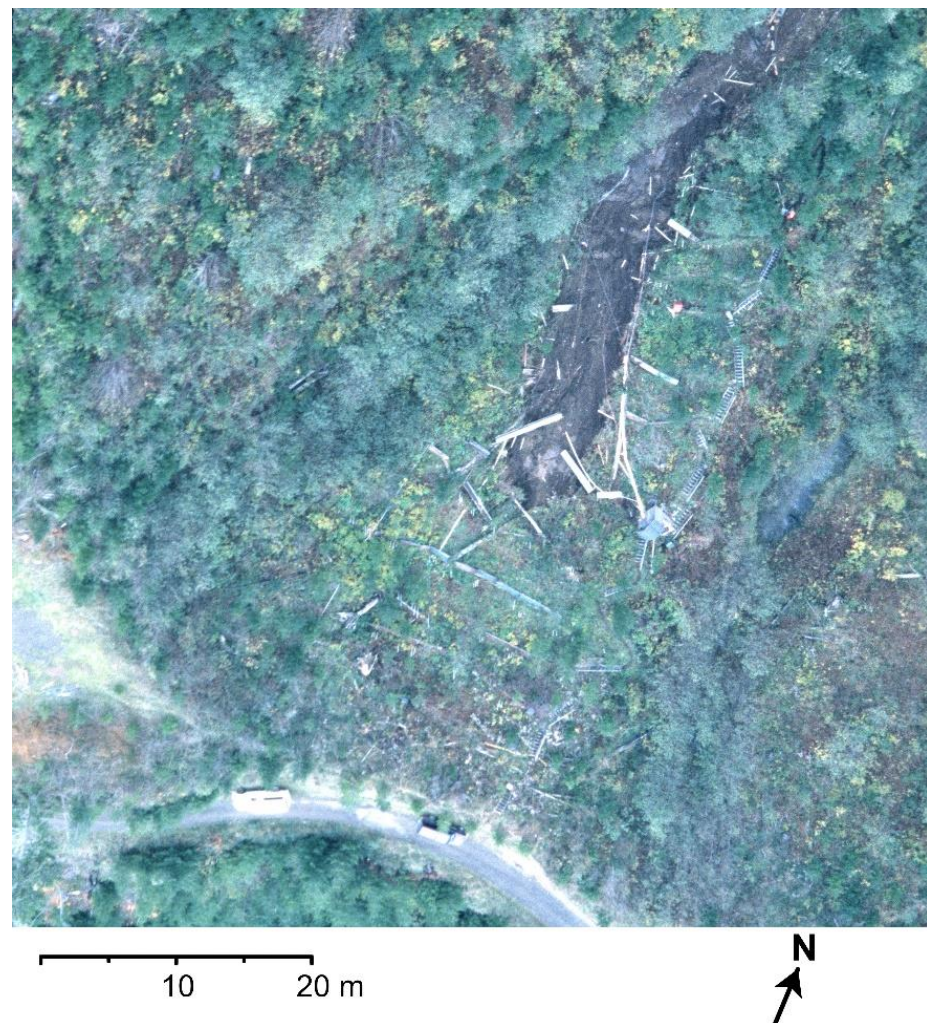
Figure 1. Post-landslide oblique aerial photo, taken roughly towards the NNW direction, reveals both upslope shallow landslide extent and downslope debris flow scour. Vehicles on the road near the bottom of the image indicate the relative size of the landslide area. Photograph by K.M. Schmidt, U.S. Geological Survey.
