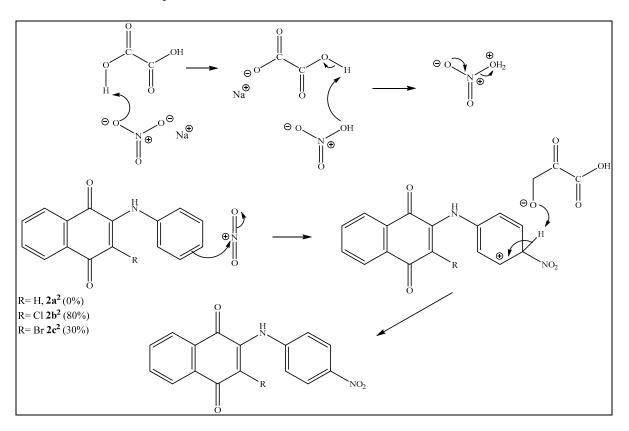
Figure 4. Solvent-free nitration of 2-anilino-1,4-naphthoquinones.
