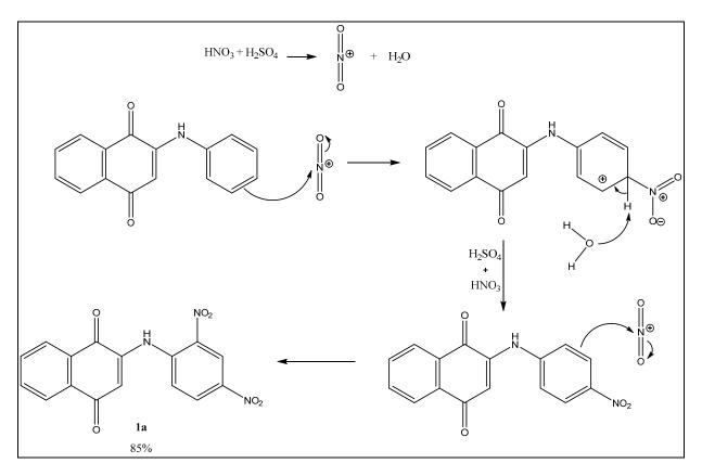
Figure 2. Mechanism classic of aromatic nitration with 1,4-naphthoquinones.
