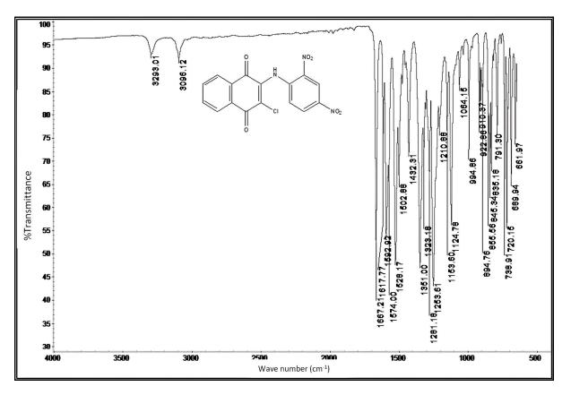
Figure 5. IR spectra of 3-chloro-2-(2,4-dinitrophenylamino)1,4-naphthoquinone.
