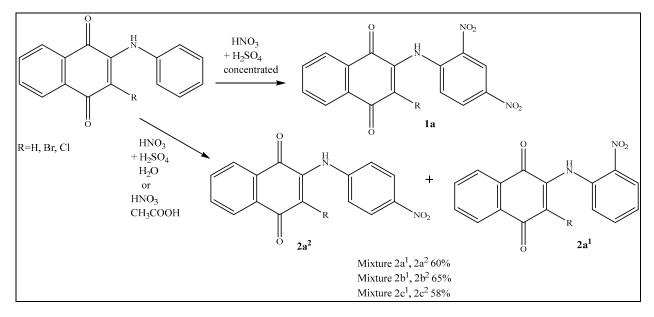
Figure 3. Di and mononitration of 3-R-(phenylamino), 1,4-naphthoquinone.
