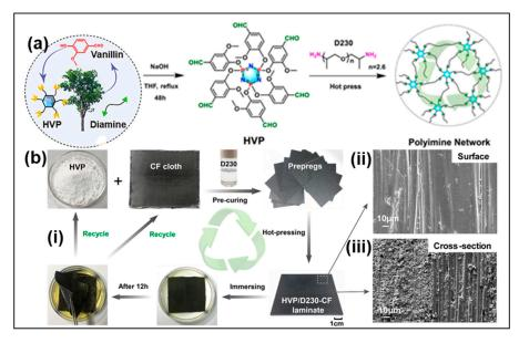
**Figure 10.** (a) Synthesis procedure of polyimine vitrimer; (b) formation of HVP/D230-CF composite and its upcycling (i), and SEM image (ii) surface and (iii) cross-section [reproduced with permission from Liu et al.; published by Elsevier, 2021] [51].
