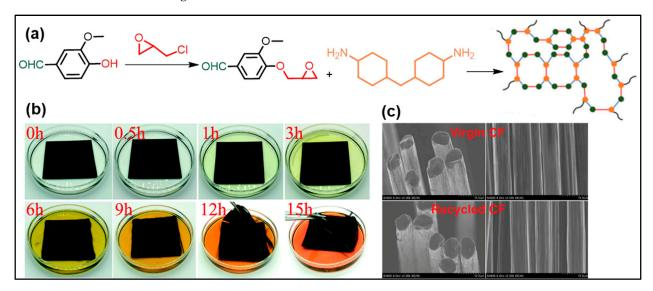
**Figure 5.** (a) Preparation way of epoxy vitrimer, (b) epoxy thermoset decomposition in 0.1 M HCl solution (methanol/ $H_2O = 8/2$ , V/V) at normal temperature for the recovery of carbon fibers from CFRCs, and its SEM images (c) [reproduced with permission from Wang et al.; published by RSC, 2019] [59].
