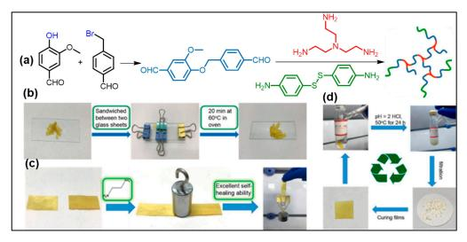
**Figure 8.** (a) Synthesis pathway of vanillin vitrimer; (b) mechanical regeneration of finely ground vitrimers; (c) self-healing performance of the cut samples that could sustain 500 g of load; and (d) chemical reprocessing of the cured vitrimers [reproduced with permission from Guo et al.; published by Elsevier, 2020] [69].
