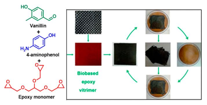
**Figure 15.** Synthesis way of vanillin-modified vitrimer and full recycling of carbon fiber reinforced composite (CFRP) [reproduced with permission from Liu et al.; published by ACS, 2021] [78].
