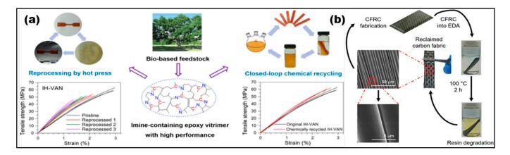
**Figure 13.** (a) Mechanically and chemically closed-loop recycling process and stress-strain curves of the cured biomass vanillin-modified themosets [18]; (b) schematic diagram of the complete reprocessing method of CFRCs and morphology of the surface of the recovered carbon fiber [reproduced with permission from Memon et al.; published by Elsevier, 2020] [80].
