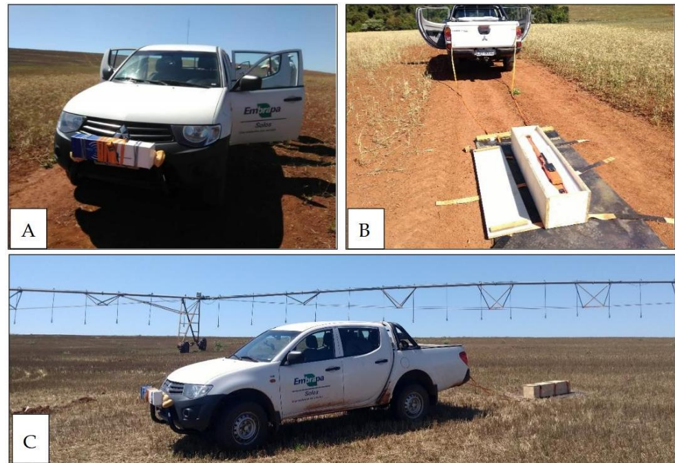
Figure 2. (A) MS1200 gamma-ray spectrometer mounted to the vehicle's brush grille guard; (B) EM38-MK2 sensor cushioned inside a wooden box mounted on a rubber mat and tied to the vehicle's rear; (C) fully equipped vehicle showing the irrigation line in the background.
