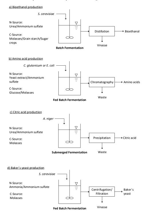
Figure 1. Flow diagrams for the production of bioethanol, amino acids, citric acid, and baker's yeast.
