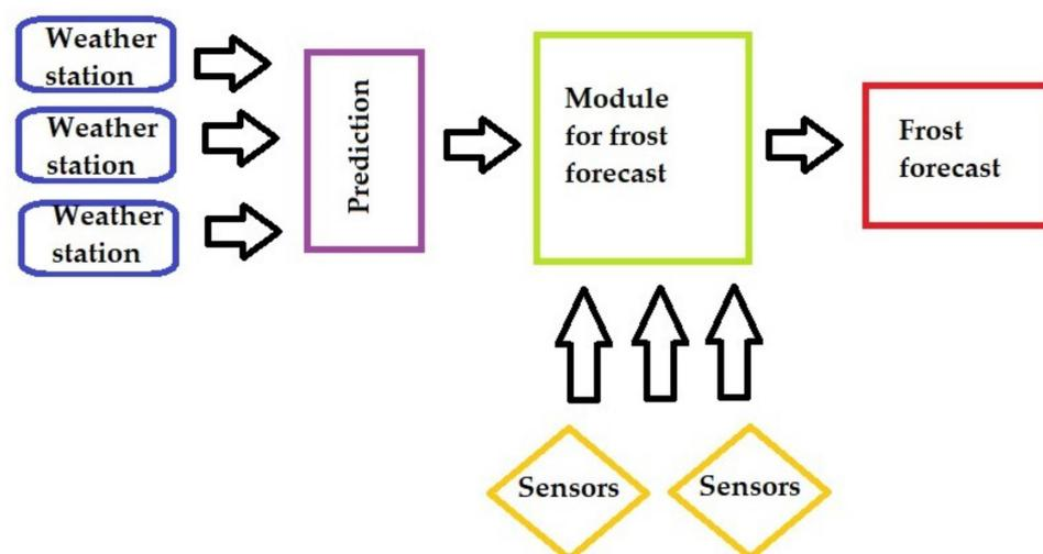
**Figure 3.** IoT-based frost prediction system.
