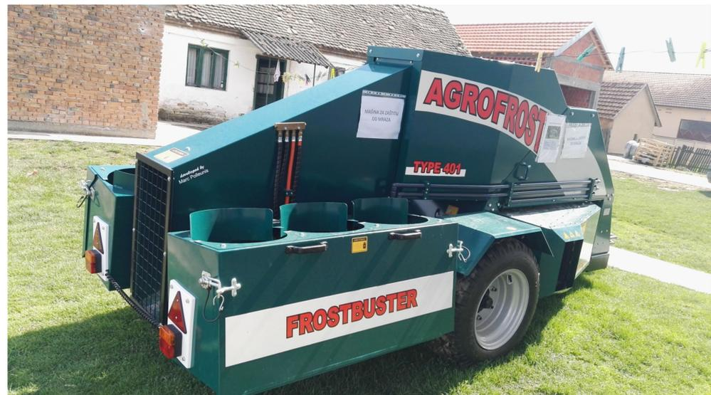
**Figure 11.** Mobile heat generator—Frostbuster.
