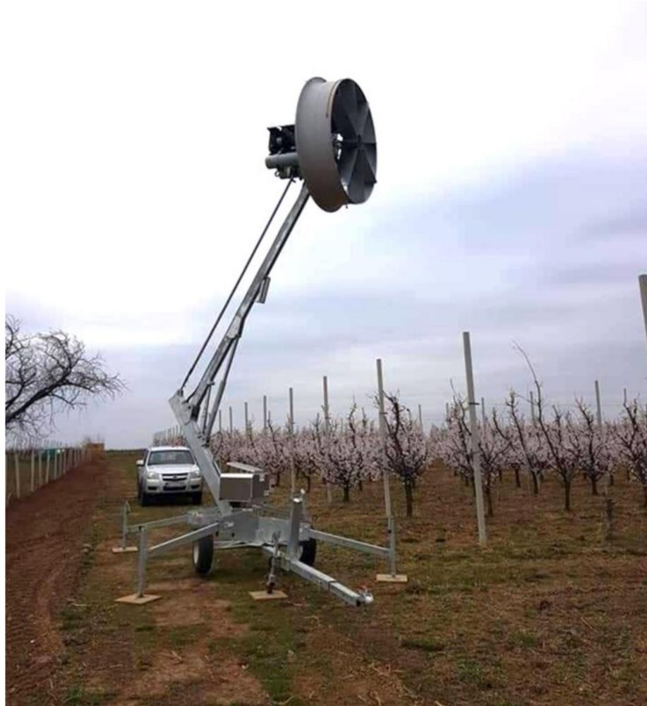
**Figure 13.** Fans for protection from spring frost.
