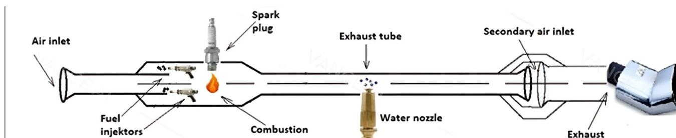
Figure 12. Schematic of a pulse-jet combustor.
