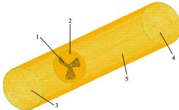
1. Impeller 2. Rotation region 3. Inlet 4. Outlet 5. Wind tunnel
