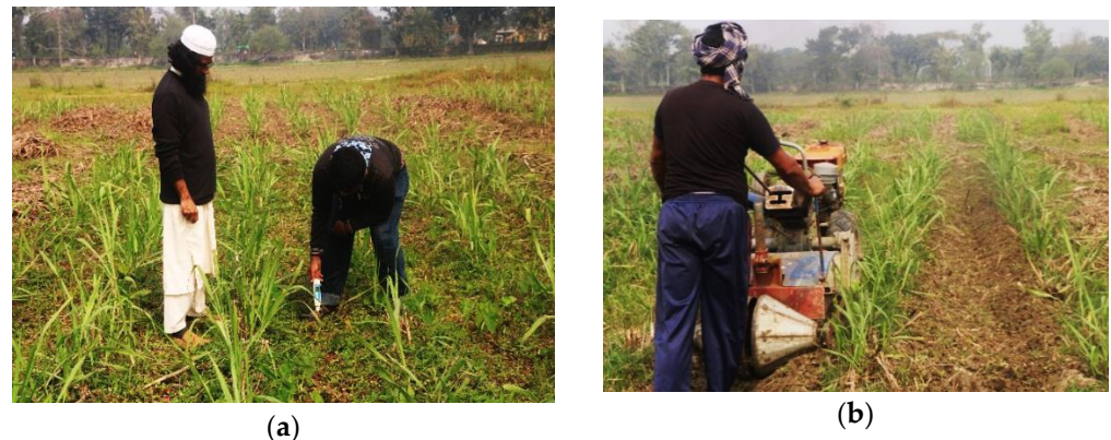
Figure 7. (a) Soil moisture measurement before earthing-up operation, (b) field test of the developed earthing-up machine.
