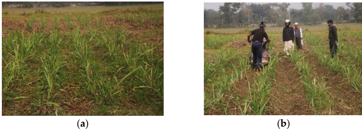
Figure 10. Field performance test of the developed earthing-up machine. (a) Sugarcane field before earthing up. (b) Earthing up with developed machine.
