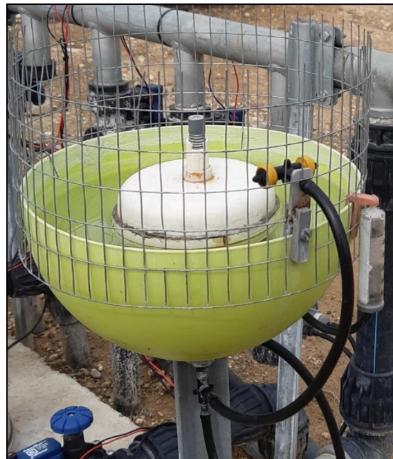
Figure 2. External tube connected to the HEM prototype for use as a water evaporated (mm) metering device.
