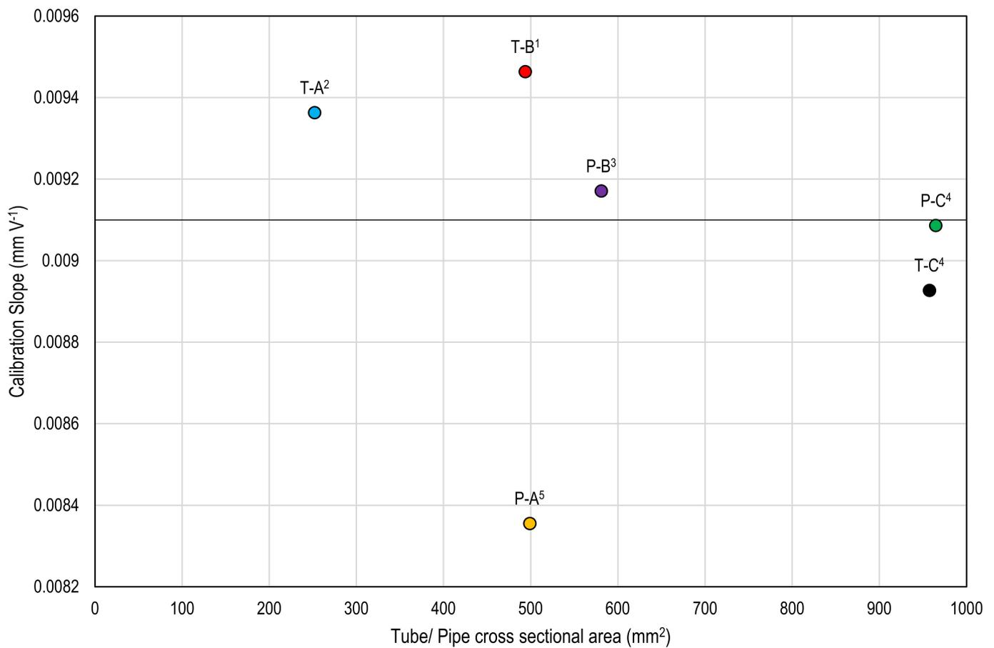
**Figure 3.** Cross-section area of tube/pipe ( $x$  axis) versus the calibration slope ( $y$  axis). Points not connected by the same letter are statistically significant,  $p < 0.05$ . The black line represents the manufacturer's provided slope.
