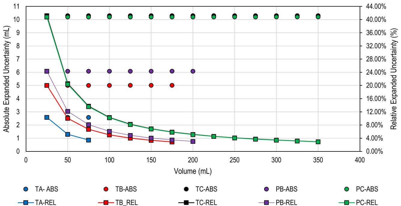
Figure 5. Absolute and relative uncertainty associated with the liquid volume measurements from each tube and pipe from the operational performance data.
