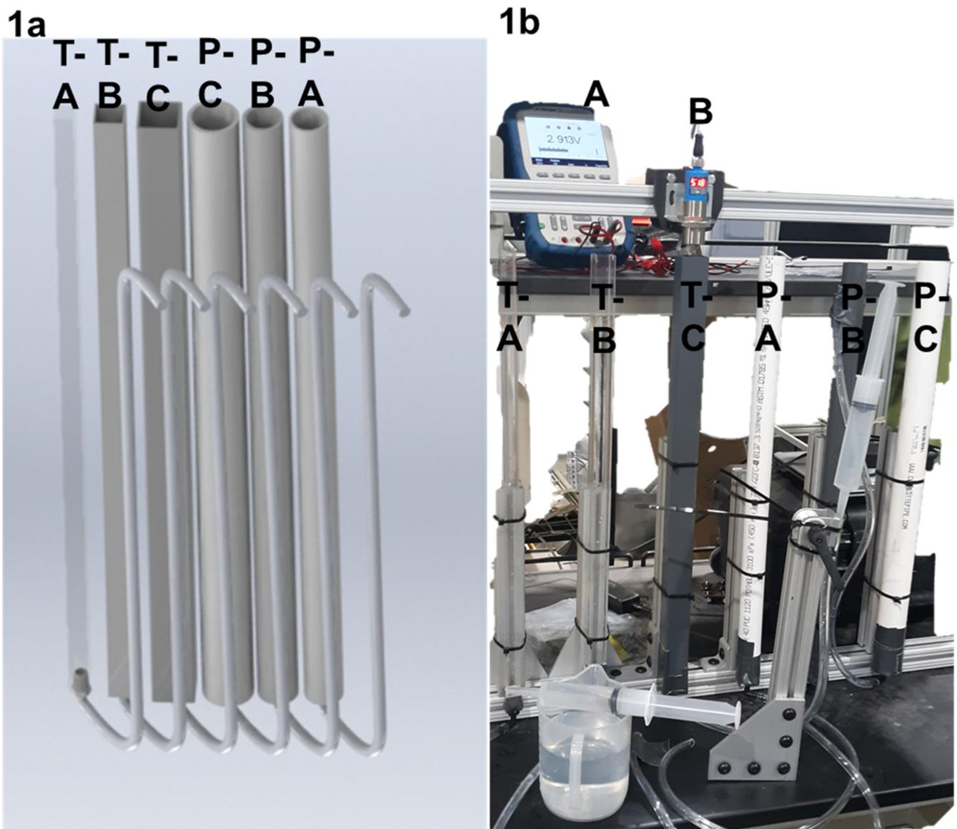
**Figure 1.** (1a) Experimental set-up sketch, (1b) picture of experimental set-up with (A) DSO and (B) ultrasonic sensor. All tubes and pipes are labeled with specifications provided in Table 1.
