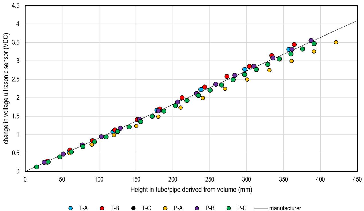
**Figure 2.** Linear regression of height of water added (x axis) vs. change in voltage from the sensor (y axis) of each tube and pipe. The black line represents the manufacturer’s calibration values.
