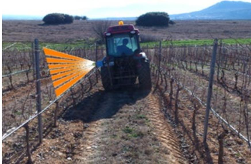
**Figure 2.** Field measurement with the LMS 200 laser scanner with a vineyard tractor.
