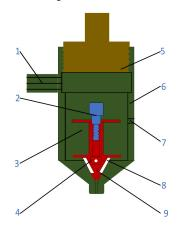
**Figure 13.** Three-dimensional cutting view of nozzle. 1: Water inlet; 2: Magnetorheological fluid cavity plug; 3: Coil winding shaft; 4: Magnetorheological fluid chamber; 5: Nozzle end cover; 6: Shell body; 7: Conductor hole; 8: Elastic cavity; 9: Swirl chamber.
