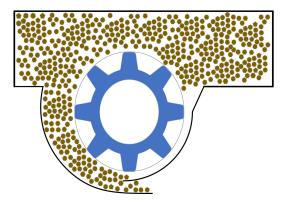
Figure 4. External grooved wheel fertilizer ejector.
