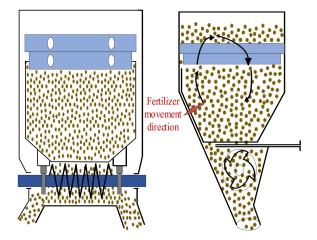
Figure 6. Centrifugal fertilizer ejector.
