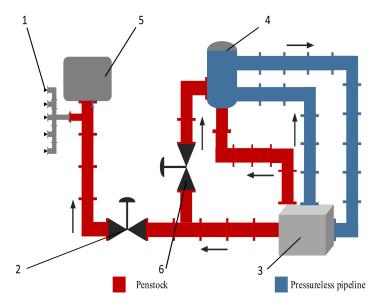
**Figure 12.** Nonlinear variable spray system. 1: Nozzle; 2: Electric on–off valve; 3: Pump; 4. Medicine box; 5: Pressure sensor; 6: Electric proportional valve. (The black arrow in the figure shows the flow direction of the aqueous solution.)
