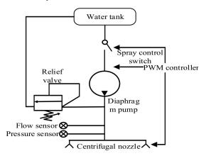
Figure 14. Composition of spray actuator.
