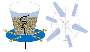
Figure 5. Centrifugal fertilizer ejector.
