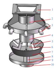
**Figure 10.** Spirally disturbed vertebral centrifugal fertilizer extractor. 1: Connecting base of fertilizer box; 2: Upper shell; 3: Fertilizer discharge pipe; 4: Spiral disturbance cup; 5: Centrifugal push plate; 6: Fertilizer room; 7: Vertebral disk; 8: Drive shaft; 9: Lower shell; 10: Bearing pedestal.
