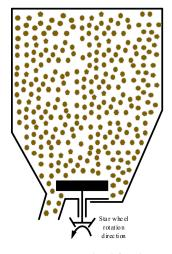
Figure 7. Star wheel fertilizer ejector.
