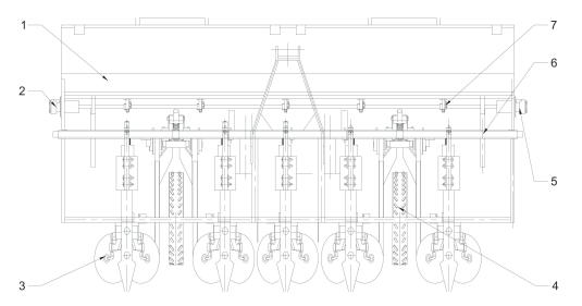
**Figure 8.** Structure of variable rate fertilization mechanism. 1: Fertilizer bin; 2: Opening motor; 3: Trenching and earth covering device; 4: Profiling wheel structure; 5: Speed motor; 6: Rack; 7: Fertilizer discharging device.
