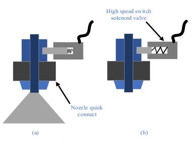
Figure 11. PWM variable nozzle. Solenoid valve on (a); Solenoid valve closed (b).
