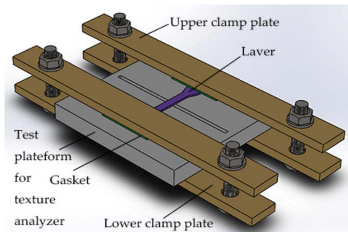
**Figure 4.** Clamp for the shear test.
