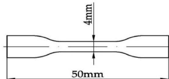
Figure 3. Samples used in tensile and shear experiments.
