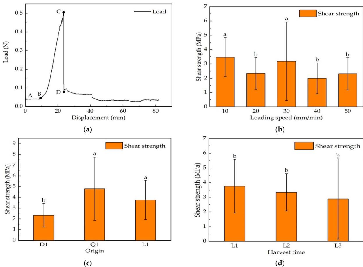
**Figure 8.** Shear properties of laver: (a) the load–displacement curve of the shear test of laver; (b) the effect of loading rate on shear strength; (c) the effect of origin on shear strength; (d) the effect of harvest time on shear strength. The different lowercase letters indicate a significant difference between groups ( $p < 0.05$ ), while same lowercase letters indicate no significant difference between groups ( $p > 0.05$ ).
