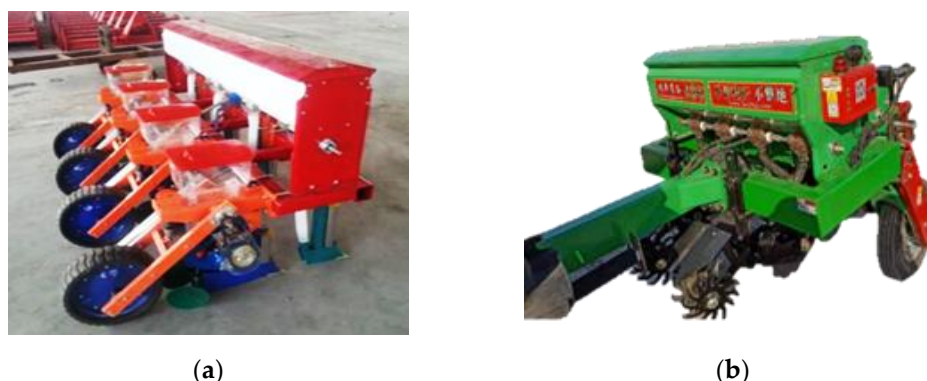
Figure 3. Examples of typical machine. (a) Huinong 2BJFG-4 no-tillage fertilization precision seeder [23]. (b) Zhaofeng 2BFM-2 no-tillage fertilizer seeder [24].
