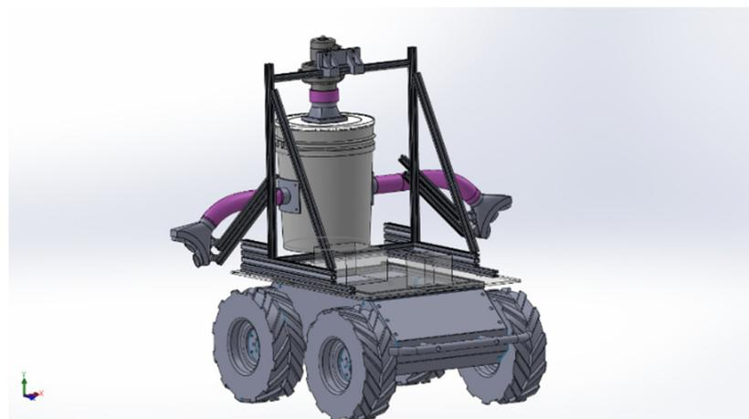
**Figure 2.** Revised design of cotton-harvesting autonomous platform (CHAP).
