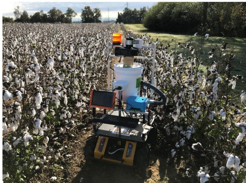
**Figure 6.** The mobile platform with the harvester module.
