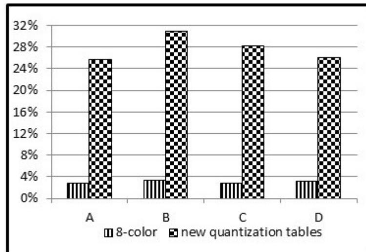
**Figure 6.** The decrease in file size in the tested images. A–D mark the images in Figures 4 and 5.
