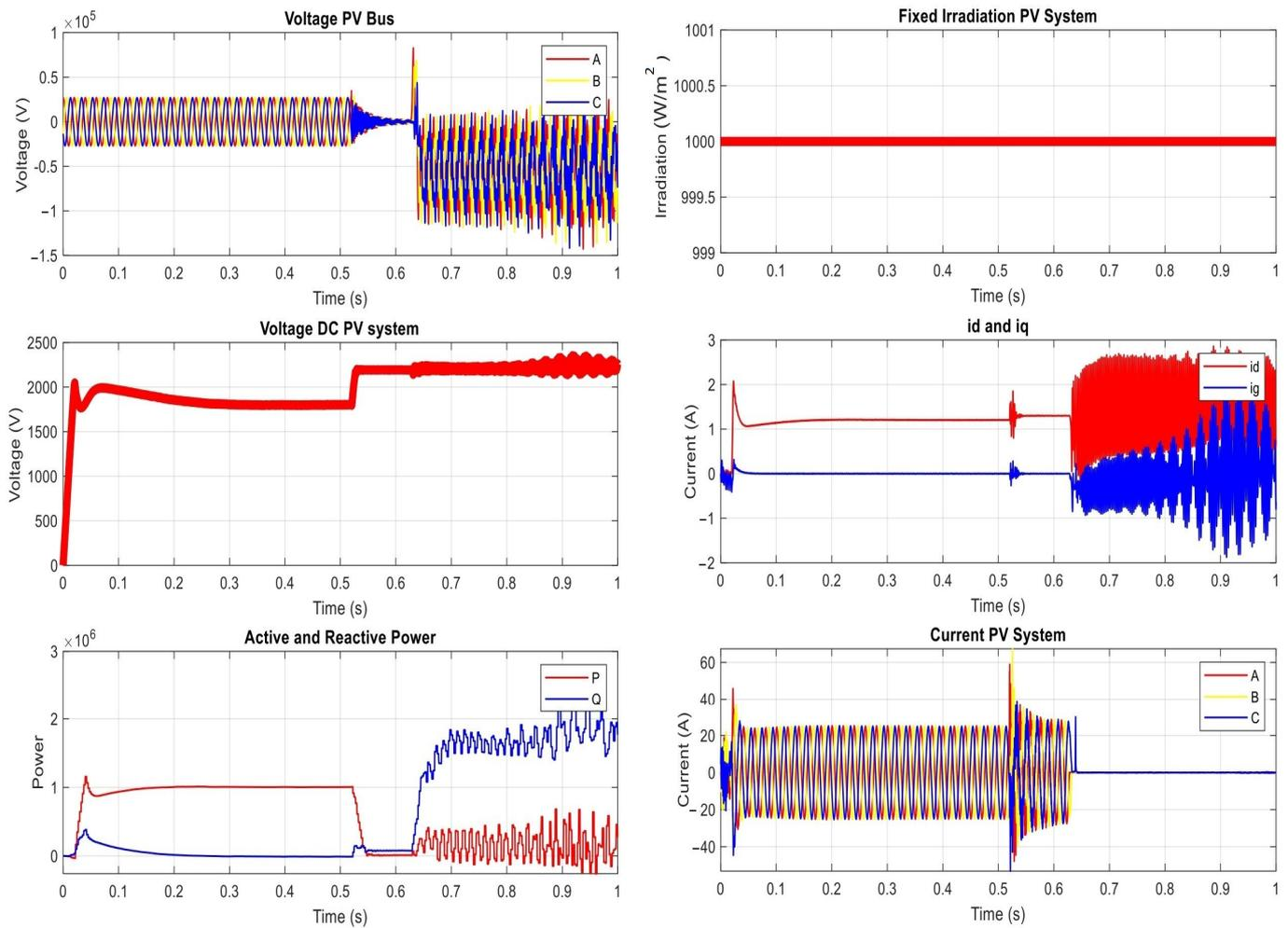
**Figure 6.** The results of the proposed power network under manipulating group settings attack on OCR.
