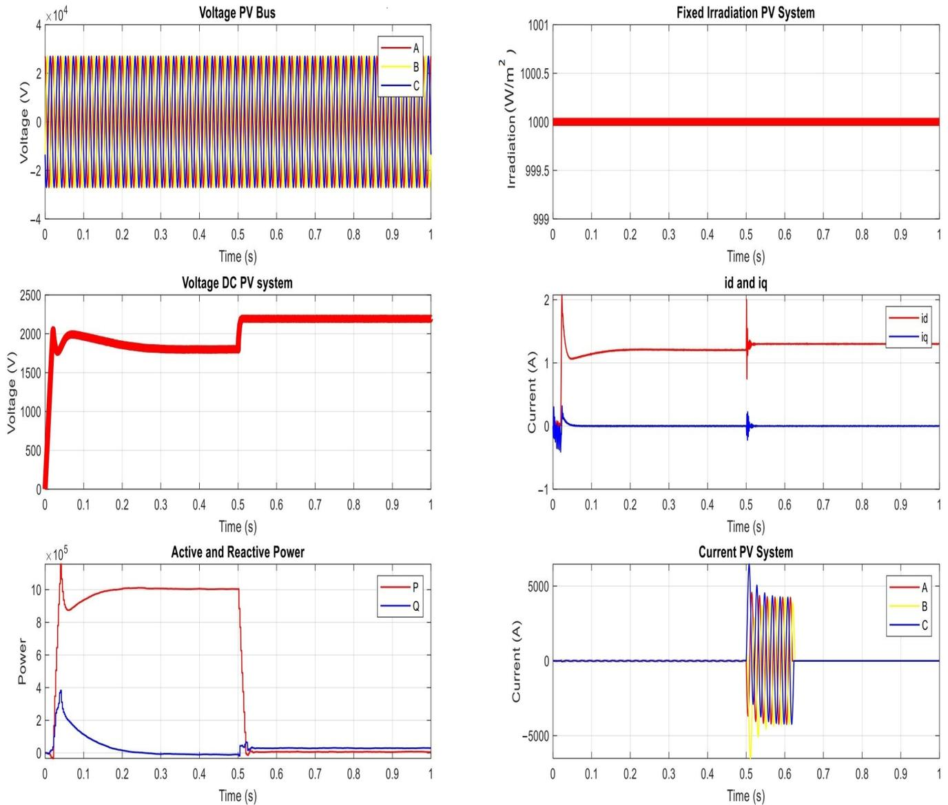
**Figure 8.** The results of the proposed power network under delaying fault messaging attack on PV farm side.
