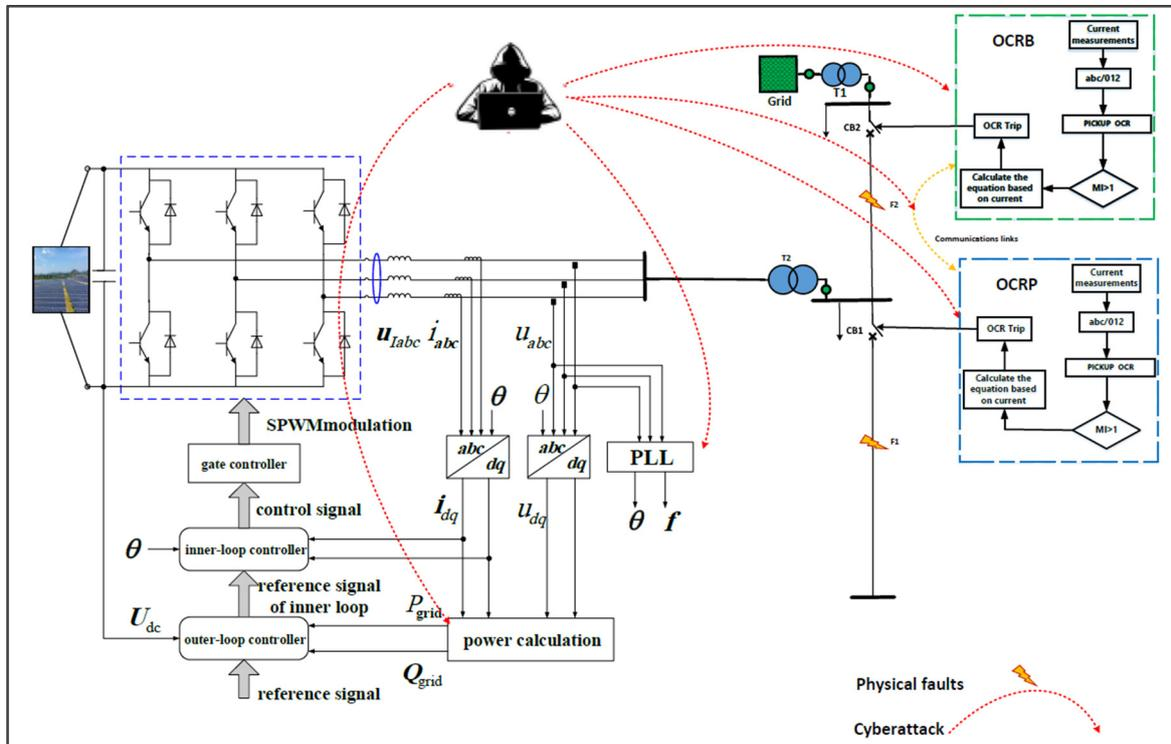
**Figure 1.** The power system configuration of grid-connected inverter and OCRs with existing physical faults and cyber threats.
