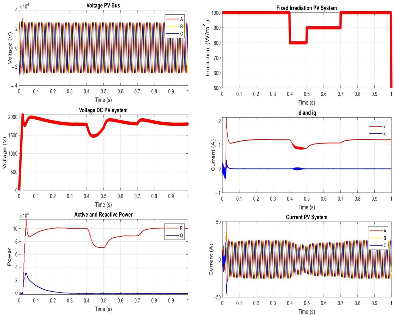
**Figure 5.** The results of the proposed power network under normal operation conditions with different levels of irradiation.
