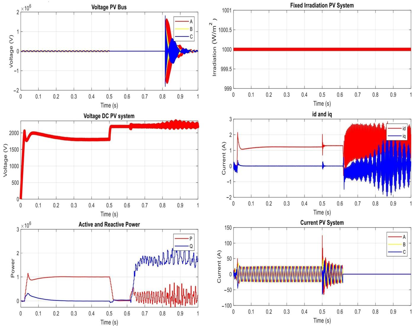
**Figure 7.** The results of the proposed power network under delaying fault messaging attack on transformer side.
