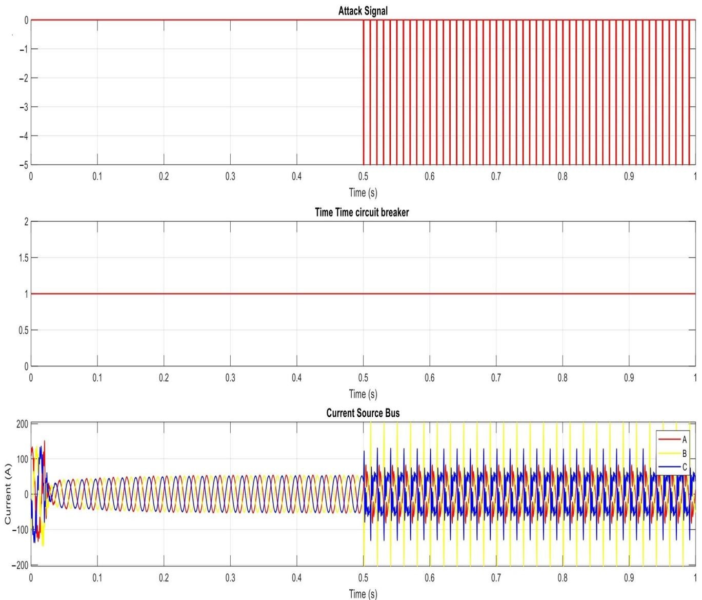
**Figure 9.** The continuous pulse signal attack on PV inverters.
