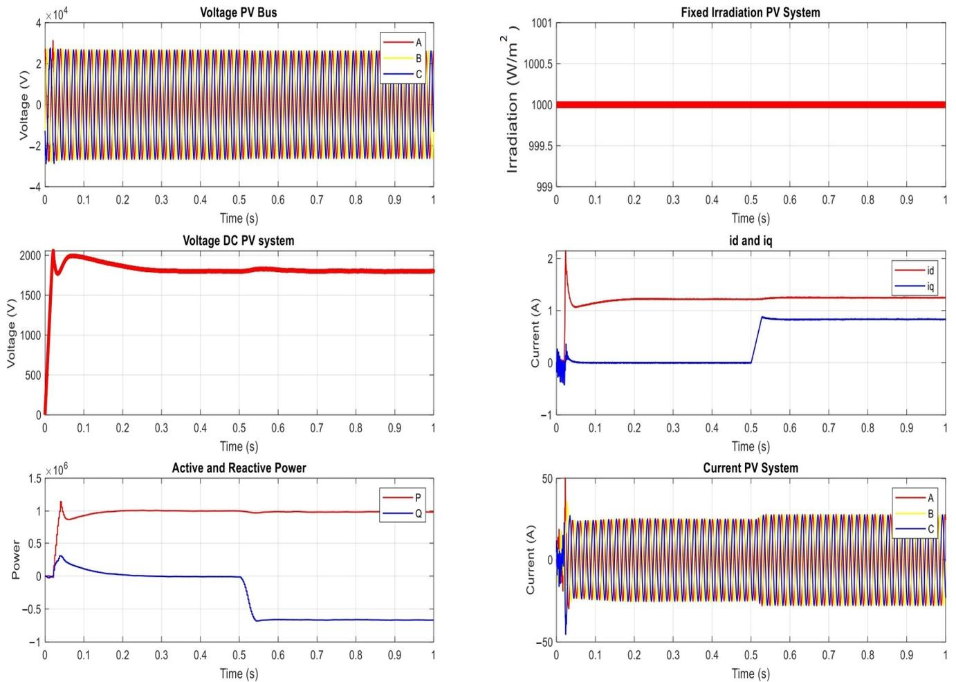
**Figure 18.** The results of the proposed power network under ramp signal attack and circuit breaker on PV inverters.
