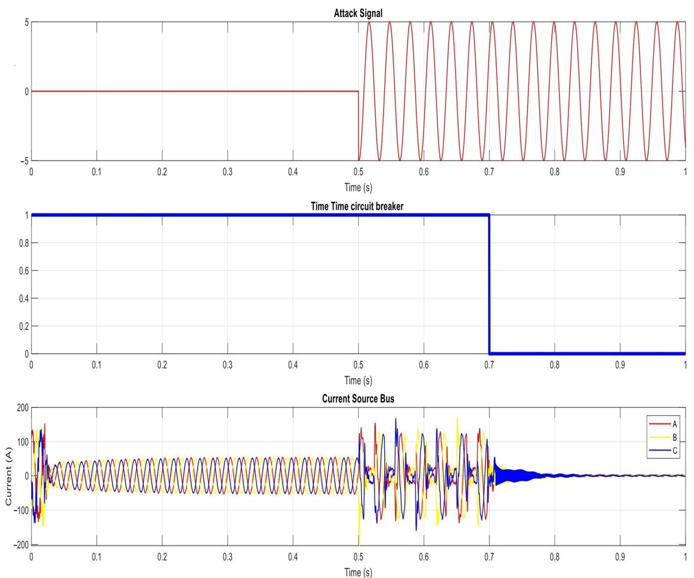
**Figure 13.** The sine signal attack on PV inverters.
