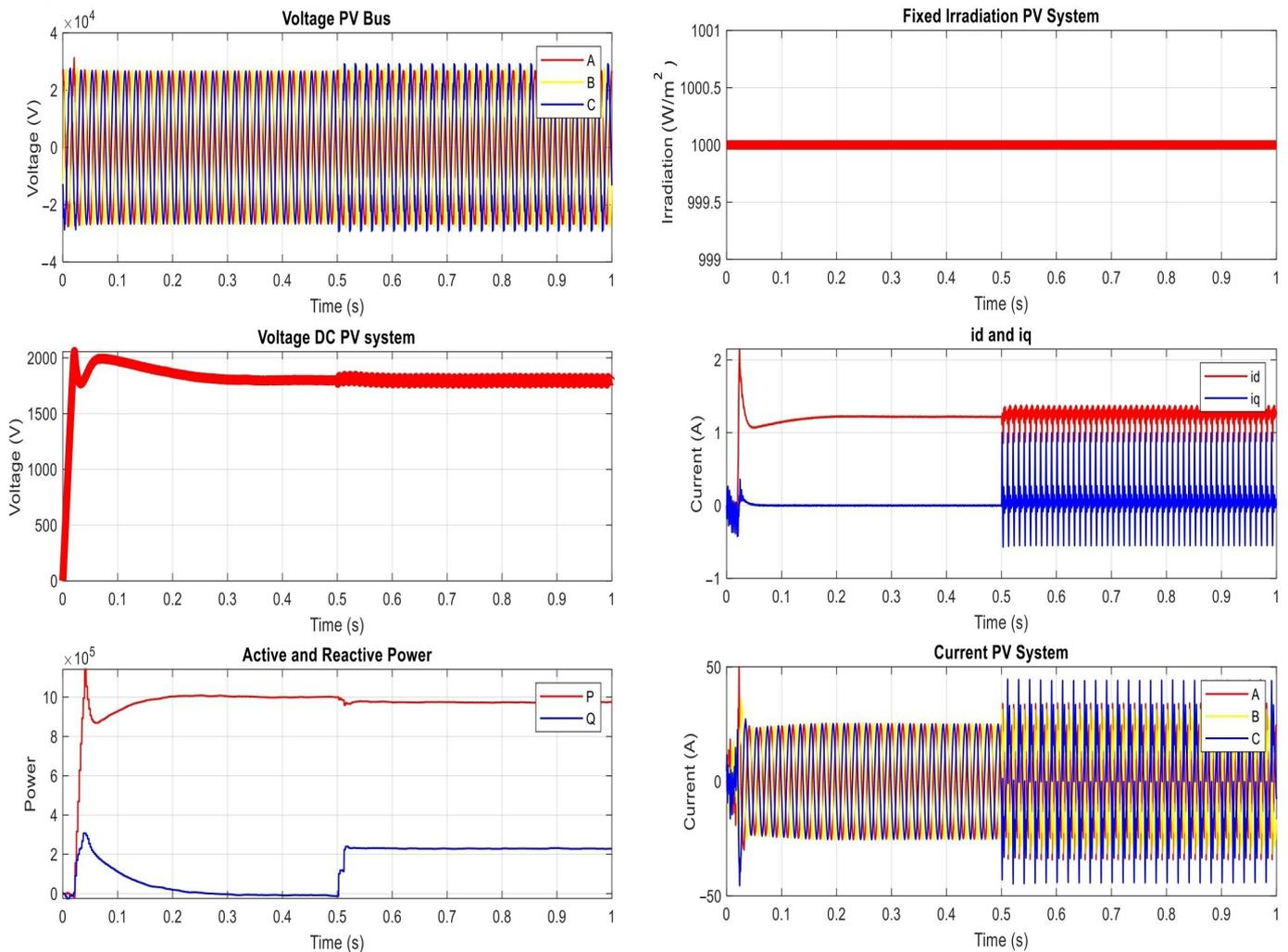
**Figure 10.** The results of the proposed power network under continuous pulse signal attack on PV inverters.
