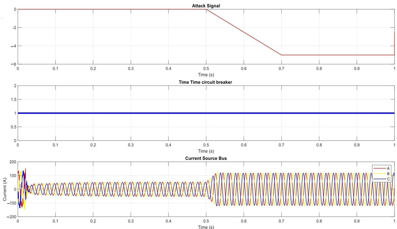
**Figure 17.** The ramp signal attack on PV inverters and circuit breaker during fault condition.
