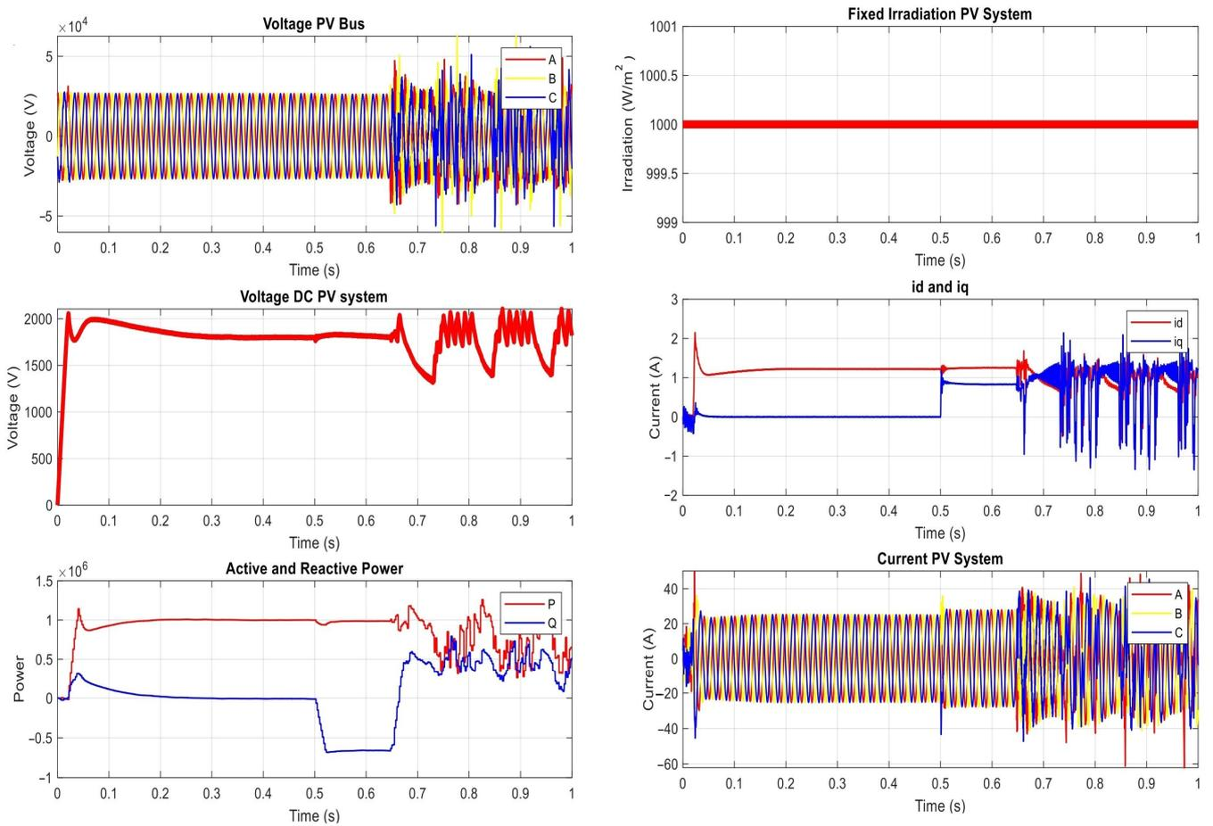
Figure 12. The results of the proposed power network under scaling signal on PV inverters.
