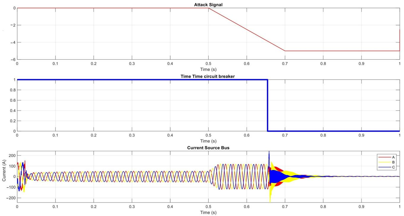
Figure 15. The ramp signal attack on PV inverters.
