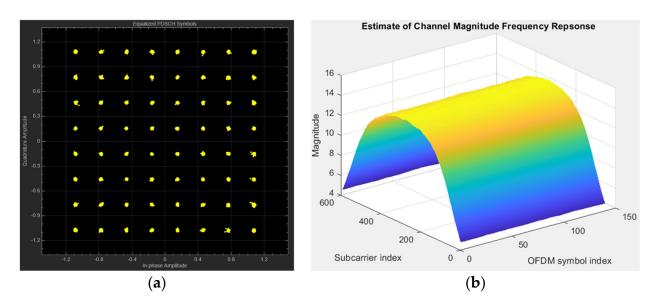
Figure 8. (a) Equalized PDSCH Symbols; (b) Channel Magnitude Frequency Response.
