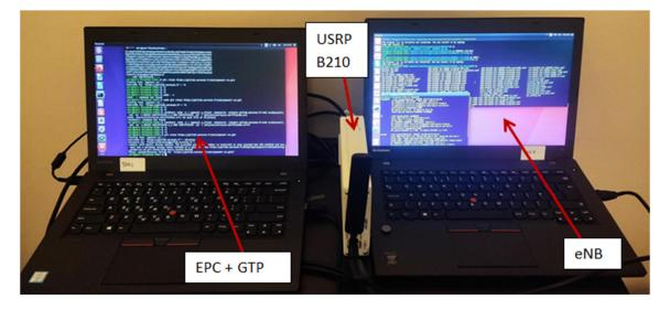
Figure 2. 4G/LTE Base Station Setup.
