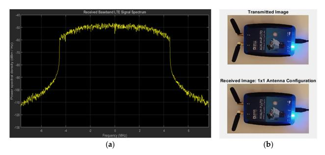
Figure 9. (a) Received Baseband LTE Signal Spectrum; (b) Transmitted and Received Image.
