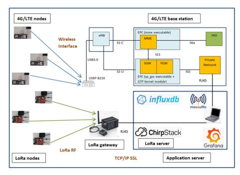
Figure 4. ECS utilized architecture and network topology.
