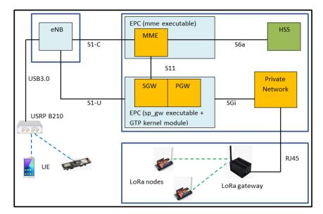
Figure 1. ECS Hybrid Approach—High-Level Architecture.
