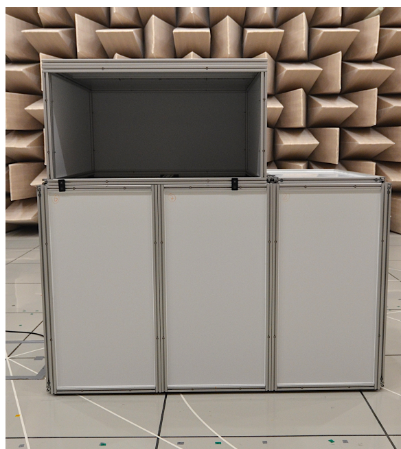
Figure 2. Photo of the model machine in the hemi-anechoic chamber in configuration II.
