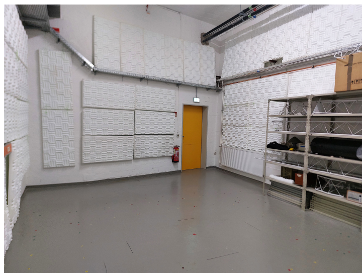
Figure 6. Former reverberation room with additional absorption at the walls and the ceiling (view in the direction of the door).
