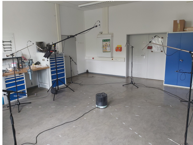
Figure 8. Photo of the workroom with the setup for the direct method to determine the equivalent absorption area.
