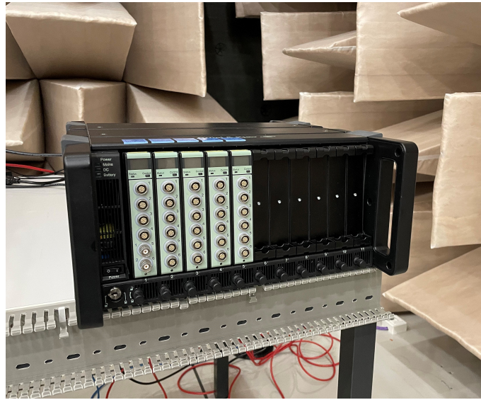
Figure A4. Photo of the Brüel & Kjaer measurement system used for the measurements.
