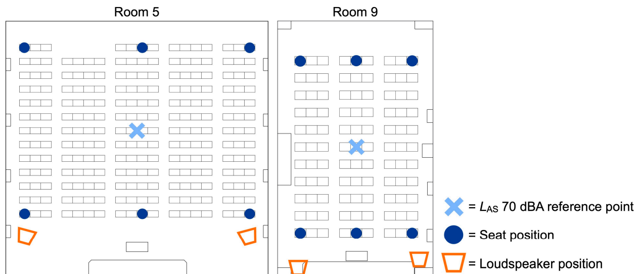
Figure 3. Seat positions and A-weighted sound pressure level set to 70 dBA at a reference point in Rooms 5 and 9.
