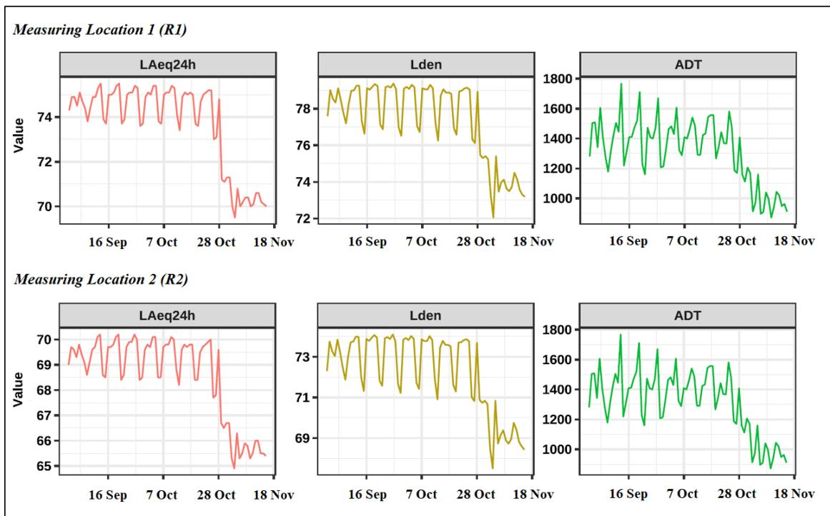
**Figure A5.** Measured noise, showing daily averages of  $L_{Aeq24h}$  and  $L_{den}$  (dBA) with the observed number of vehicles per day on the E45 motorway. Note: measurements period = 1 September–15 November 2019 ( $N = 76$  days).
