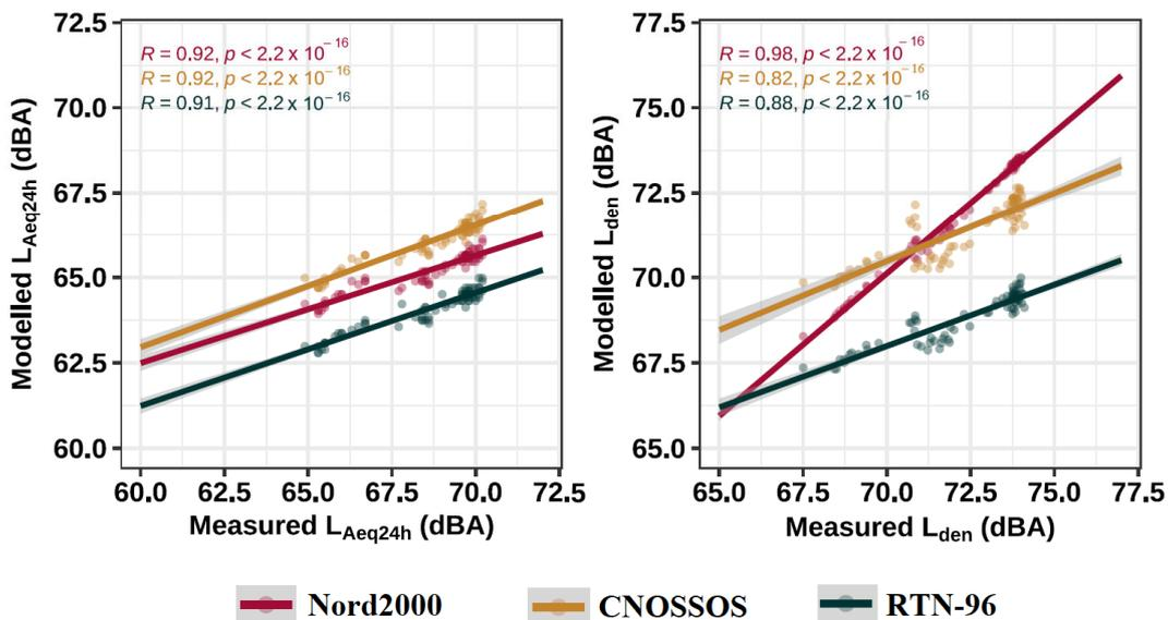
Figure 3. Comparison of the measured and modeled noise of Nord2000, CNOSSOS and RTN-96 at the two measuring locations in the study site, Helsted, Denmark. The noise levels,  $L_{Aeq24h}$  and  $L_{den}$  (N = 76 days) (daily averages), are in dBA. Note:  $R$  = Spearman’s correlation coefficient ( $R_S$ ),  $p$  =  $p$ -value showing the statistical significance of the correlation coefficients. Regression lines with 95% confidence intervals are also shown in the scatter plots.
