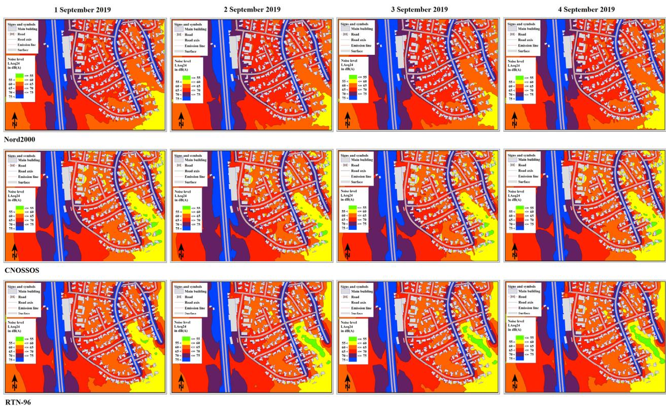
**Figure 4.** High-resolution mapping ( $5\text{ m} \times 5\text{ m}$ ; 1–4 September 2019) of  $L_{Aeq24h}$  (dBA) levels produced by Nord2000, CNOSSOS and RTN-96 in the SoundPLAN software version 8.2. Maps of 1–4 September 2019 are shown here. See Figure A6 for the maps of 5–7 September 2019.
