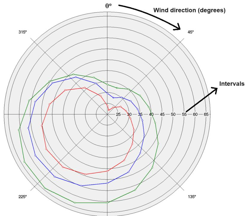
**Figure A3.** Schematic representation of the share of CNOSSOS' favorable sound propagation for the day (07:00–19:00; red color), evening (19:00–22.00; blue color) and nighttime (22.00–19.00; green color) in Denmark. The schematic shows wind direction from 0 to 360 degrees. The above schematic is taken from the CNOSSOS “DK Weather” library in the SoundPLAN software version 8.2.
