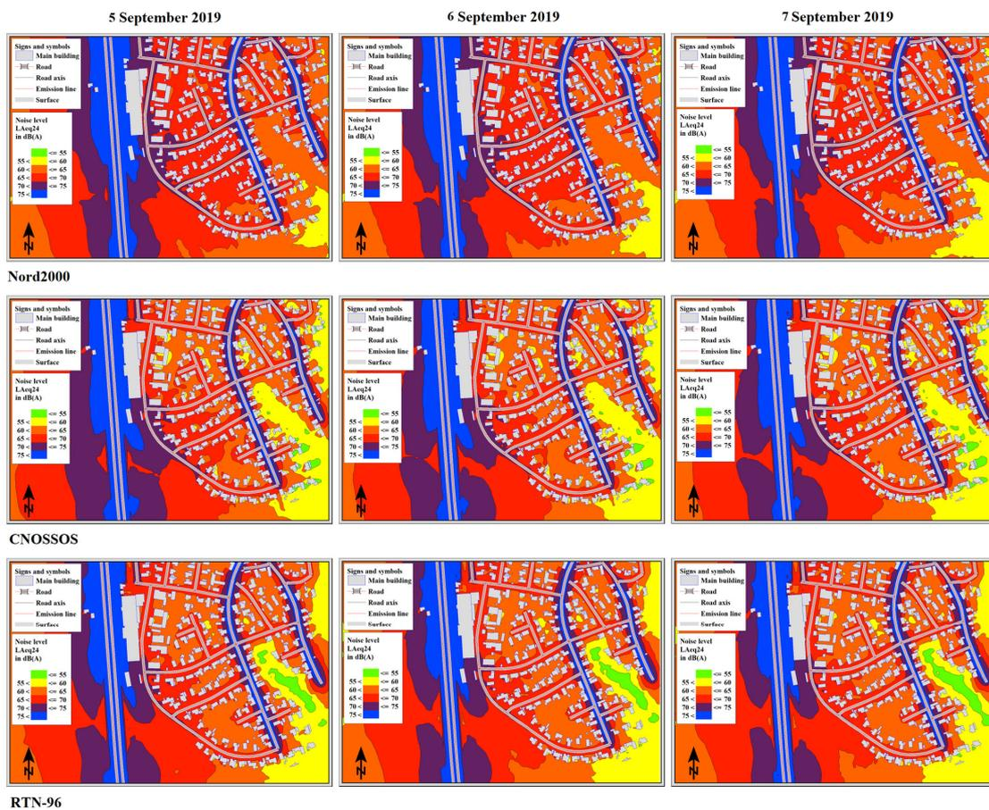
**Figure A6.** High-resolution maps (5 m × 5 m) of estimated  $L_{Aeq24h}$  (dBA) levels of Nord2000, CNOSSOS and RTN-96 in Helsted, Denmark for 5–7 September 2019.
