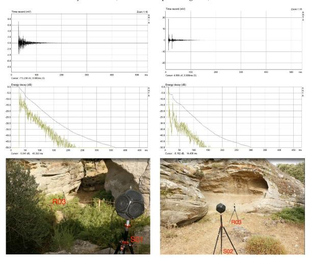
**Figure 5.** Impulse response (IR) and its early decay curve (EDC) captured at Bacinete main shelter with the source placed in front of the paintings (S1) and the receiver in the "audience" area (R3) (left column); and at Bacinete III, with the source in the middle of the audience area (S2) and the receiver next to the paintings (R3) (right column).
