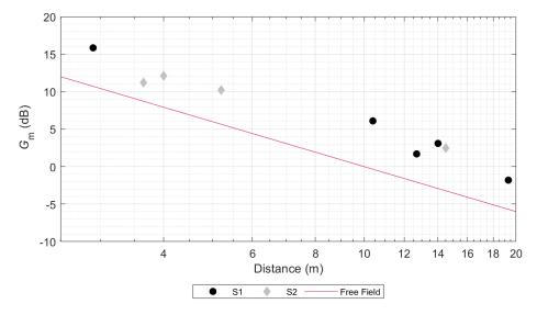
**Figure 8.** Sound strength,  $G_m$  (dB), spectrally averaged values calculated from the measured IR in the Bacinete main shelter. The theoretical free field propagation is represented by the red line.
