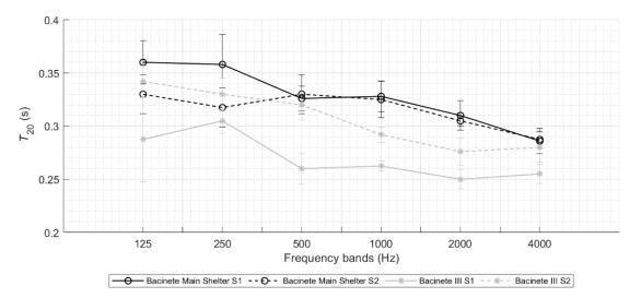
**Figure 6.** Reverberation time ( $T_{20}$ ) obtained in each shelter of the Bacinete rock art complex: Bacinete main shelter; Bacinete III. Spatially averaged values for each source location are represented at each frequency band.
