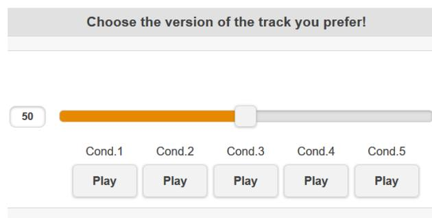
**Figure 6.** Graphical user interface of the experimental procedure. Cond.1–Cond.5 correspond to the differently processed versions of the same song. The slider bar corresponds to the volume.
