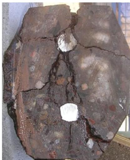
**Figure 3.** Colour-enhanced and sharpened-focus photograph in 2008 of saw-cut cross-section of reinforced concrete handrail likely made in 1968, showing very low volume of rust around the steel bars and extensive cracking [21].
