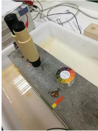
**Figure 9.** Photo showing the liquid leached out through the surface open crack in the course of the accelerated corrosion test. pH value of the liquid: 2 to 3.
