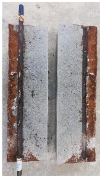
**Figure 10.** Photos showing the appearance of the split parts of an RCM specimen broken after finishing the accelerated corrosion test. The surfaces of the open crack reaching the upper surface are fully coated with the typical reddish-brown corrosion products of steel, while the region below the steel bar is free from corrosion products.
