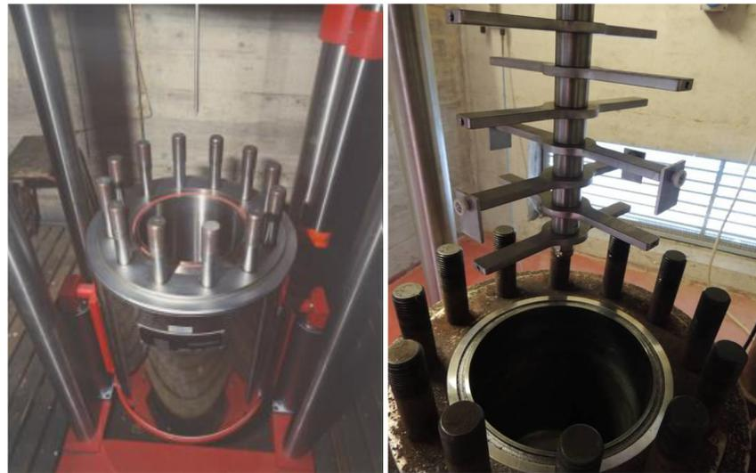
**Figure 1.** Autoclave (20 L) for corrosion testing with the water stirring apparatus.
