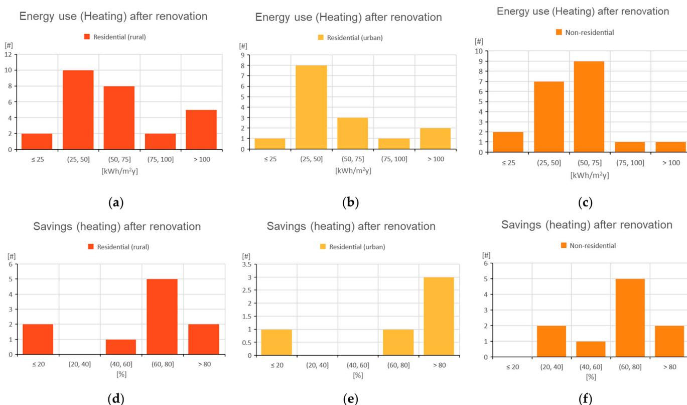
**Figure 9.** Energy use for space heating (in kWh/m<sup>2</sup>y) (a–c) and energy savings (in %) (d–f) according to building use (residential rural, residential urban, and non-residential).
