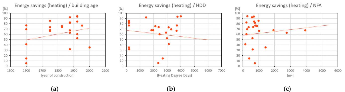
**Figure 8.** Energy savings (in %) in terms of space heating demand ( $n = 25$ ) as a function of (a) building age ( $R^2 = 0.05$ ), (b) Heating Degree Days ( $R^2 = 0.02$ ), and (c) Net Floor Area ( $R^2 = 0.01$ ).
