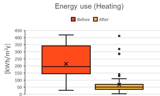
**Figure 6.** Energy use for space heating in kWh/m<sup>2</sup>y before and after retrofit ( $n_{\text{before}} = 26$ ,  $n_{\text{after}} = 62$ ).
