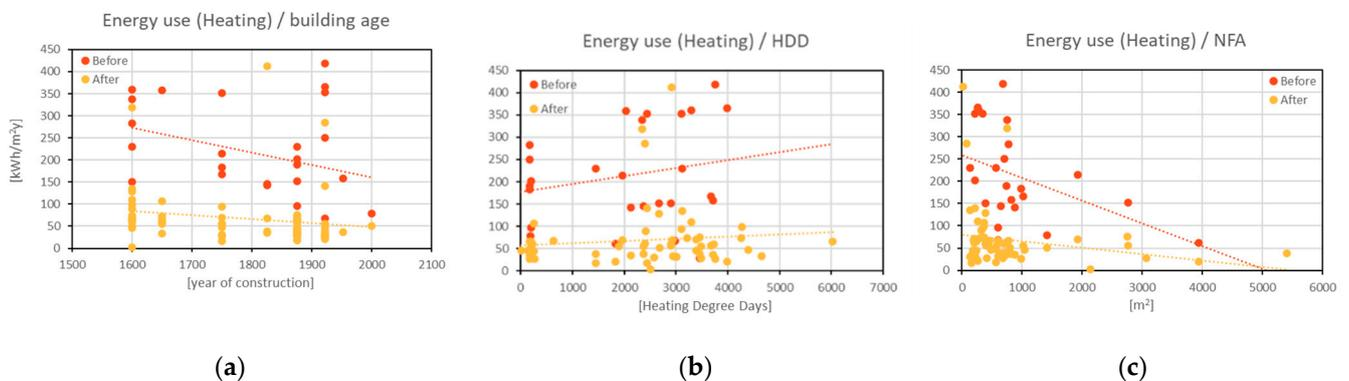
**Figure 11.** Energy use (in kWh/m<sup>2</sup>y) before and after retrofit as a function of (a) building's age ( $R^2$ before = 0.11,  $R^2$ after = 0.03), (b) Heating Degree Days ( $R^2$ before = 0.05,  $R^2$ after = 0.01), and (c) Net Floor Area ( $R^2$ before = 0.16,  $R^2$ after = 0.04).
