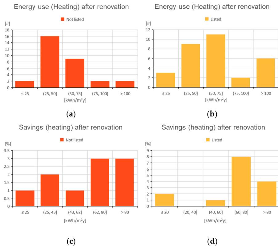
**Figure 10.** (a,b) Energy use for space heating in kWh/m<sup>2</sup>y and (c,d) energy savings in % for listed and not listed buildings.
