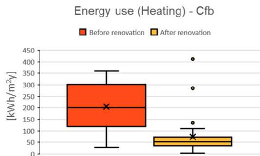
**Figure 7.** Energy use for space heating in kWh/m<sup>2</sup>y before and after retrofit in climatic zone Cfb.
