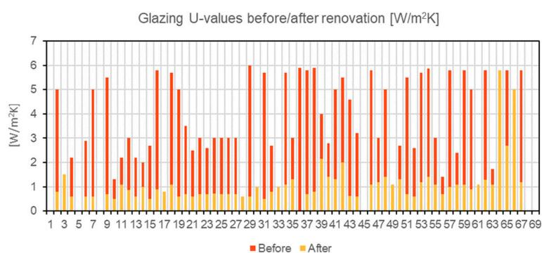
**Figure 1.** Window glazing U-values before and after renovation.
