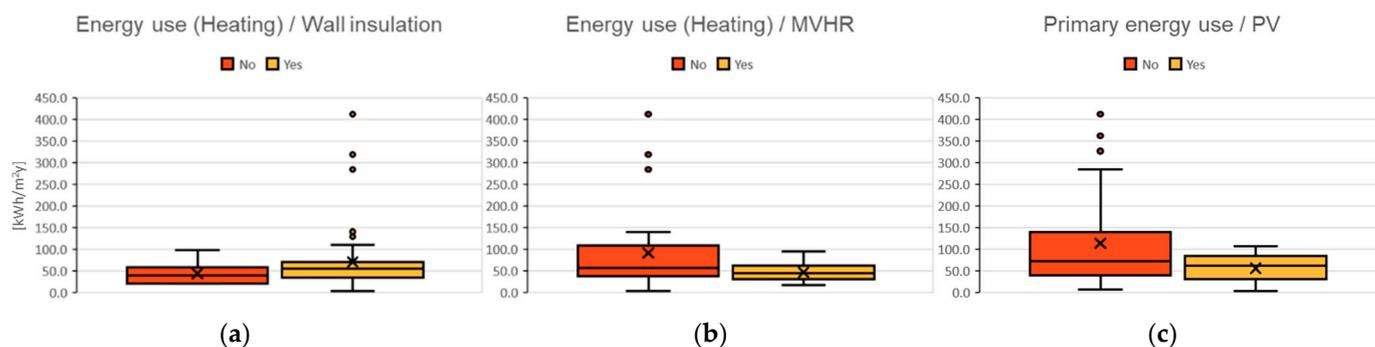
**Figure 12.** Energy use (in kWh/m<sup>2</sup>y) after retrofit according to implementation of (a) wall insulation and (b) MVHR (sample size from left to right  $n = 6, 56, 30, 32$ ) and (c) total primary energy use (in kWh/m<sup>2</sup>y) in cases with and without PV systems ( $n = 34, 12$ ).
