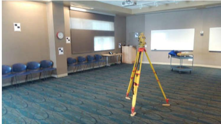
**Figure 1.** Coordinating reference targets using the total station.
