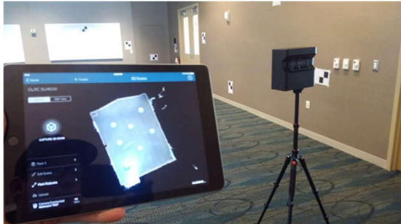
**Figure 4.** Test field surveying by the Matterport Pro camera.
