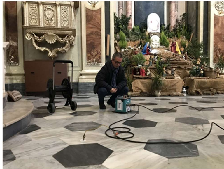
Figure 3. Phases of ERT measurements with the electrocardiogram electrodes (photo by Leucci).
