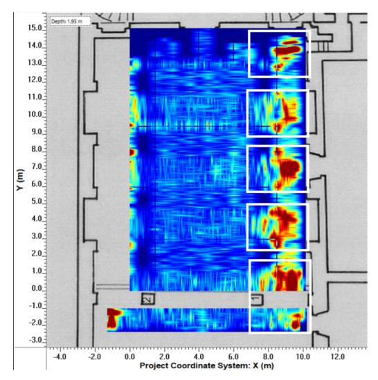
**Figure 6.** In the depth slice, at a depth of approximately 2 m, five elongated anomalies (highlighted in white) can be observed beneath the floor of the left lateral nave. These anomalies are of substantial size and appear to correspond to artificial foundations similar to those present beneath the right lateral nave, which are also visible from the exterior of the church.
