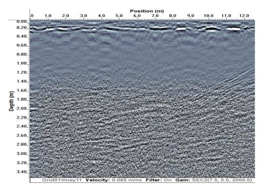
**Figure 3.** Example of a radargram acquired in the central nave where a uniform natural stratigraphy is present.
