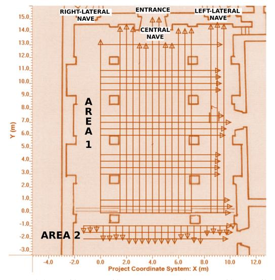
**Figure 2.** The location of the two areas of the GPR acquisitions and the orientation of the GPR profiles. Note that the squares on the map indicate the location of the column bases inside the church.
