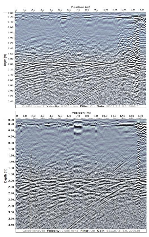
**Figure 4.** Example of two parallel radargrams acquired in the left lateral nave where a more complex anthropic stratigraphy is present at a depth of approximately 2 m. Note that, above this presumably anthropogenic structure, there is a layer of soil upon which the church floor rests, which clearly attenuates the electromagnetic signal.
