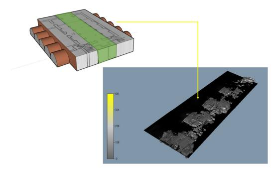
**Figure 8.** Reconstruction (on the top-left) of the possible symmetrical and vaulted anthropic spaces (highlighted in brown) built to support the church at a depth of approximately 2 m, based on the pseudo-three-dimensional reconstruction of the corresponding anomalies (on the right). In the center of the top-left reconstruction, the area beneath the central nave is highlighted in green, presumably composed of a natural tuff rock block.
