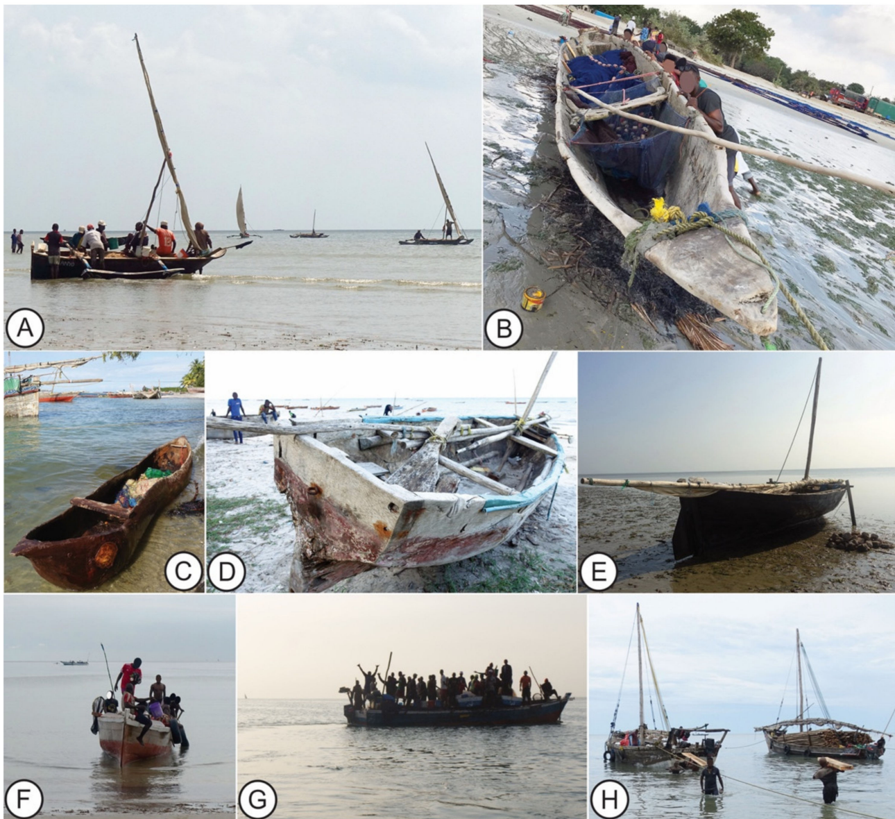
Figure 4. The working watercraft ‘heritage’ of Bagamoyo: (A) the common double-outrigger ngalawa fishing logboat; (B) a large mtumbwi fishing logboat, being careened; (C) a one-person Nyasa mtumbwi ; (D) an elaborate mashua ndogo ‘logboat’; (E) a double-ended mchoro fishing boat, which is increasingly scarce for its dependence on sail; (F) a motorised ngwanda , ferrying crew to a boti la mtando ; (G) a purse-seining boti la mtando , getting under way to fishing grounds; (H) two cargo mashuas , one being loaded with planks, the other with a cargo of eucalyptus poles. (Images: Lucy K. Blue, John P. Cooper, Javern Aveline Sabas).
