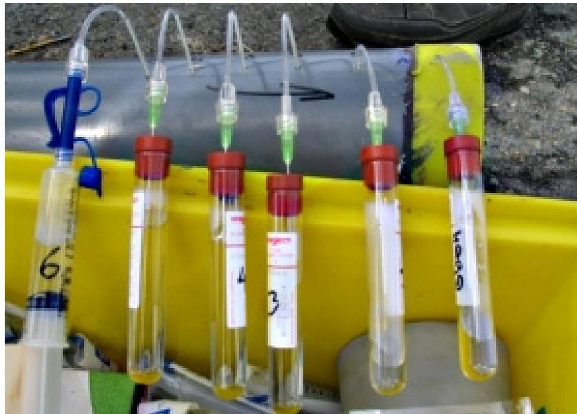
**Figure 5.** Rhizon pore water samplers, which filter pore water from the core using a blood-sampling vacuum tube.
