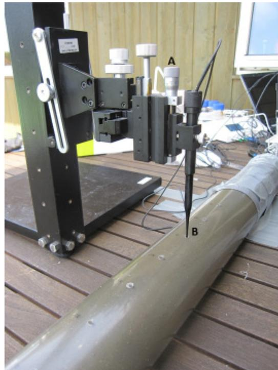
**Figure 4.** Profiling cores with sulfide sensor. A: Micromanipulator enabling insertion of microsensor. B: 500  $\mu\text{m}$  tipped sulfide sensor
