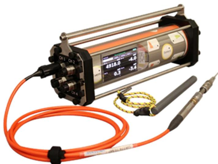
**Figure 2.** Data logger for characterizing environmental parameters in sediments. The logger has four channels and was developed to measure sulfide, pH, redox potential and dissolved oxygen.
