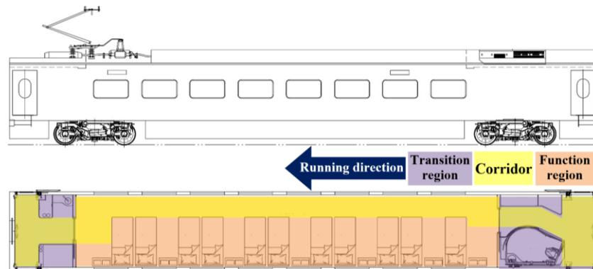
**Figure 12.** Carriage No. 6 of the high-speed sanitary train: spatial layout of the minor injury care compartment.
