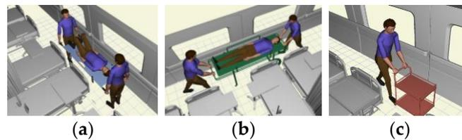
**Figure 27.** Simulation analysis of aisle trafficability of serious injury carriage. (a) The scene of walking in the carriage. (b) Manually push a two wheeled lifting stretcher to walk inside the carriage; (c) The scene of a hand propelled medical vehicle walking inside the carriage.
