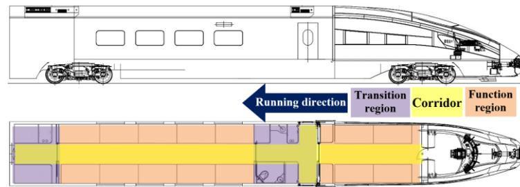
**Figure 14.** Carriage No. 8 of the high-speed sanitary train: space layout of the sleeping carriage.
