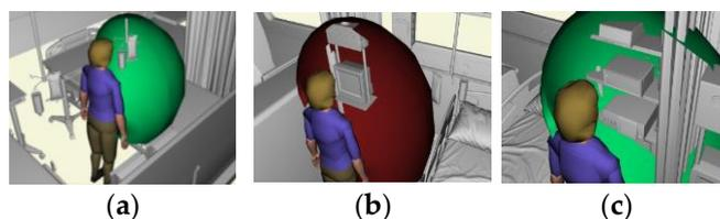
**Figure 28.** Simulation analysis of the operation of related instruments in the serious injury carriage. (a) Accessibility range for operating small bottles in front of the hospital bed; (b) P5 female digital person is operating the button. (c) The reachable range of female digital humans when operating buttons.
