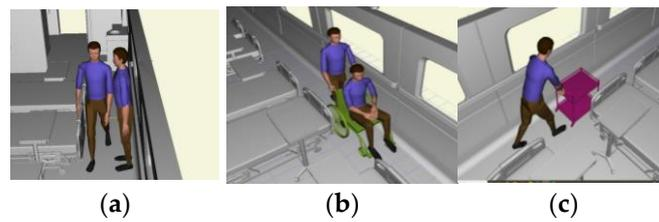
**Figure 29.** Simulation analysis of aisle trafficability of minor injury carriage. (a) The scene where two male digital figures meet in the hallway; (b) Hand propelled wheelchair scene; (c) Pushing a medical handcart in the hallway.
