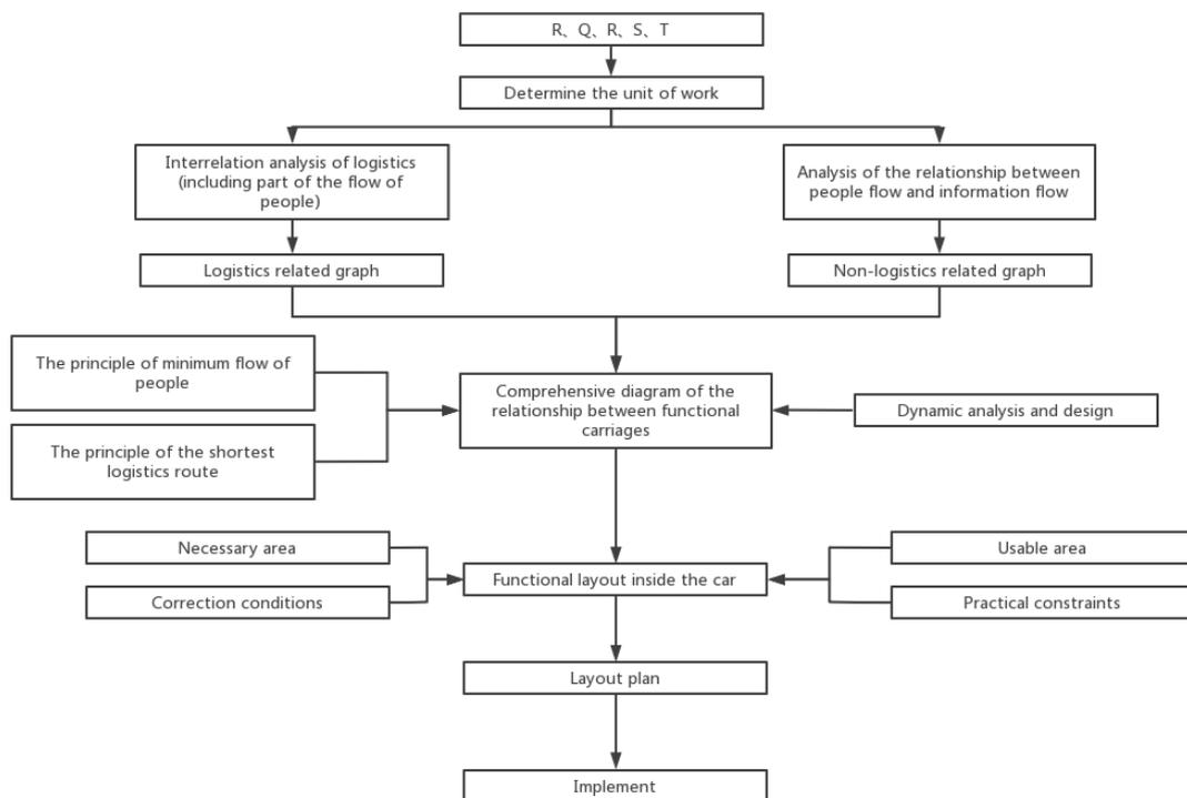
**Figure 1.** Planning model of carriage composition and interior layout of the high-speed sanitary train based on improved SLP method.
