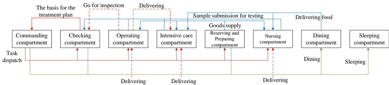
**Figure 6.** Comprehensive diagram of the mutual relationship between functional carriages of high-speed sanitary trains.
