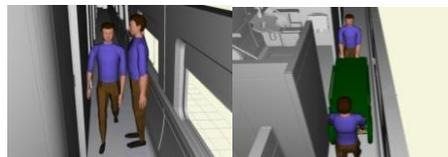
**Figure 23.** Simulation analysis of trafficability of the surgical carriage aisle.
