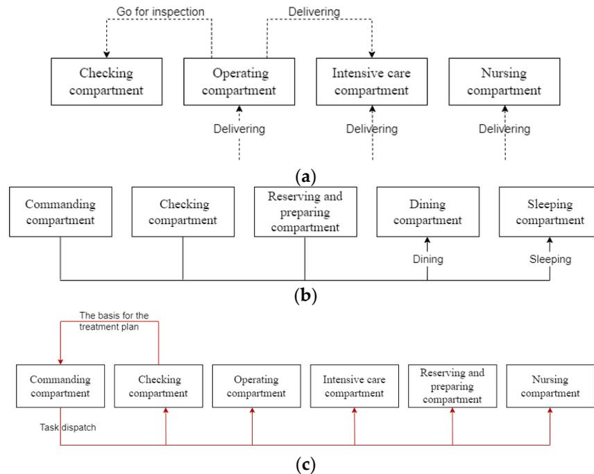
**Figure 3.** Non-logistics relationship of high-speed sanitary trains. (a) Movement of the wounded and sick. (b) Flow lines of medical staff (except logistics). (c) Information flow.
