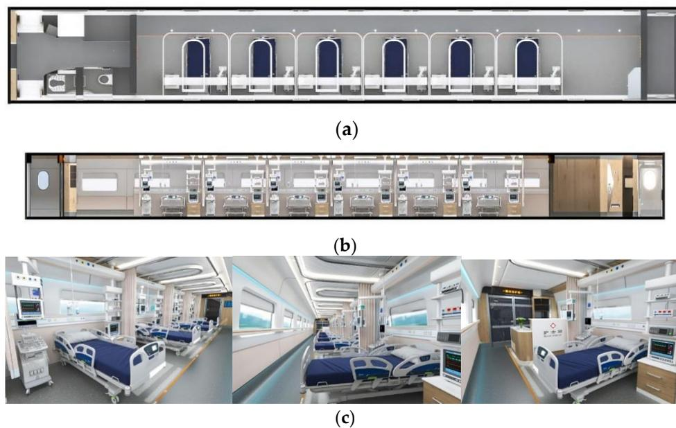
**Figure 17.** Rendering of the intensive care compartment of the high-speed sanitary train. (a) Plan of the intensive care compartment of the high-speed health train. (b) Elevation of the intensive care compartment of the high-speed sanitary train. (c) View of the intensive care compartment of the high-speed sanitary train.
