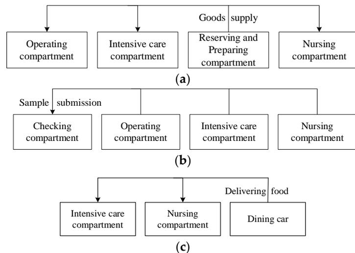
**Figure 2.** Logistics relationship of high-speed sanitary trains. (a) Logistics relationship between reserve and preparation carriages, intensive care carriages, and nursing carriages (b) Logistics relationship between surgical carriages, intensive care carriages, nursing carriages, and inspection carriages (c) The logistics relationship between dining carriages, intensive care carriages, and nursing carriages.
