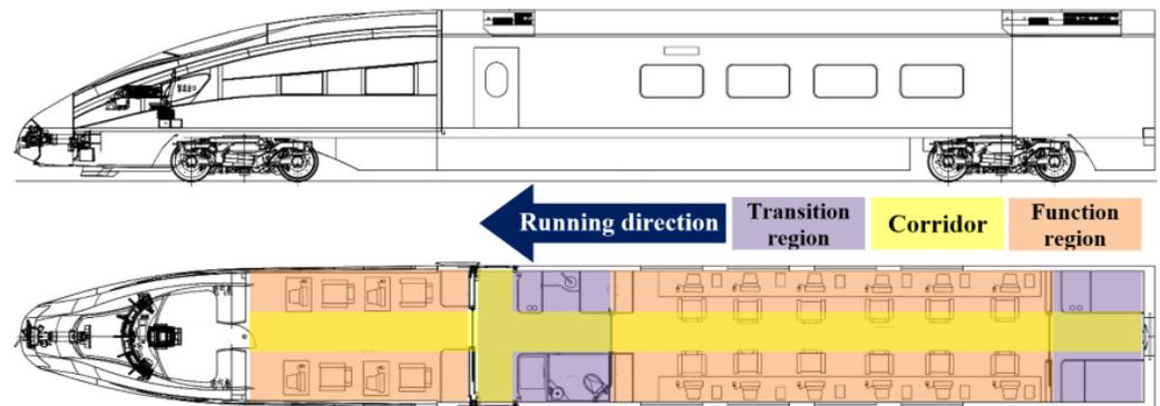
Figure 7. Carriage No. 1 of the high-speed sanitary train: spatial layout of the command compartment.
