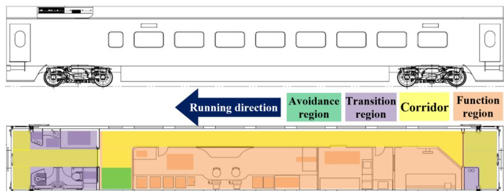
Figure 8. Carriage No. 2 of the high-speed sanitary train: space layout of the inspection carriage.
