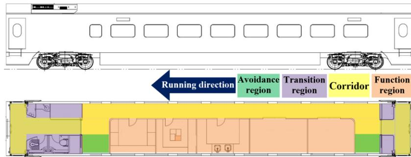
**Figure 11.** Carriage No. 5 of the high-speed sanitary train: space layout of the reserve and preparation carriage.
