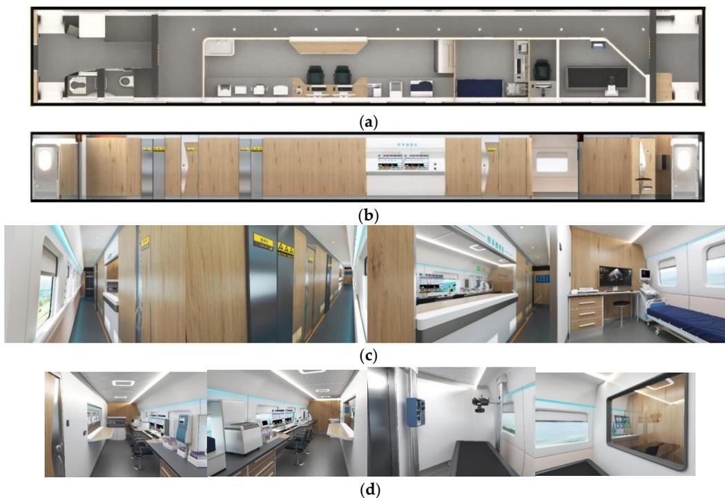
**Figure 15.** Effect drawing of the inspection compartment of the high-speed sanitary train. (a) Plan of the inspection compartment of the high-speed sanitary train. (b) Elevation view of the corridor of the inspection compartment of the high-speed sanitary train. (c) View of the corridor of the inspection carriage, the sample receiving station, and the echocardiography laboratory. (d) View of the comprehensive inspection room, ray room, and ray control room of the inspection compartment.
