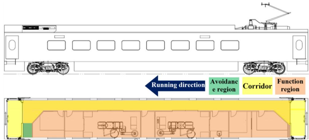
Figure 9. Carriage No. 3 of the high-speed sanitary train: spatial layout of the surgical compartment.
