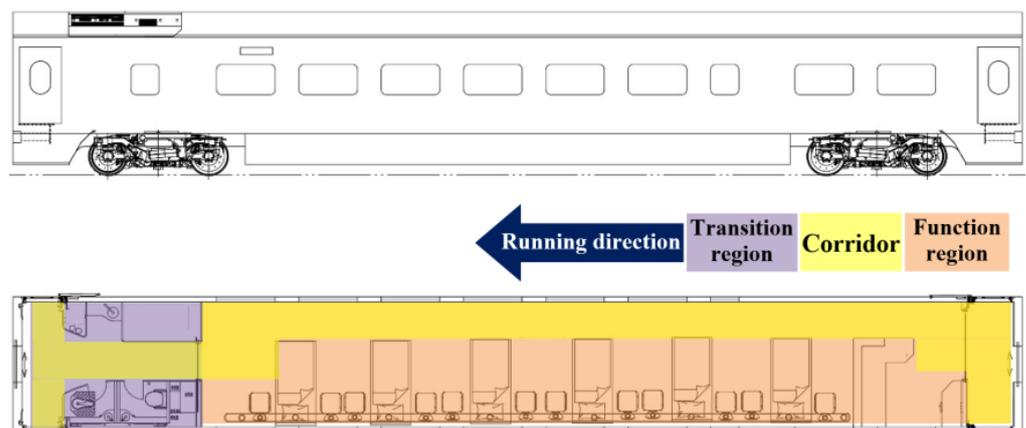
Figure 10. Carriage No. 4 of the high-speed sanitary train: space layout of the critical illness compartment.
