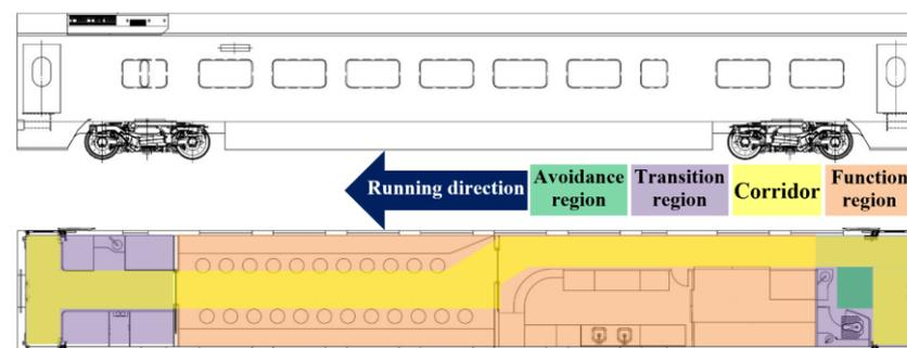
**Figure 13.** Carriage No. 7 of the high-speed sanitary train: dining car spatial layout.
