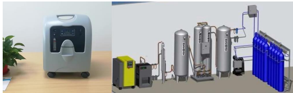
Figure 3. Portable medical oxygen PSA concentrators ( left ) and PSA oxygen concentrator plant medical oxygen generator ( right ) (Source: SPI).
