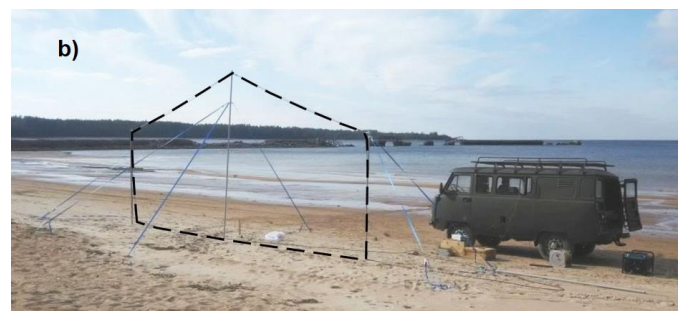
Figure 2. (a) sketch of a pentagonal loop used for realizing HMD; (b) view of the HMD layout during the field experiment. The loop is highlighted with a black dashed line.
