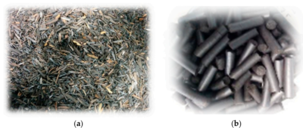
Figure 1. Photos of black spruce residues transformed into (a) biochar at 320 °C and (b) biochar pellets.
